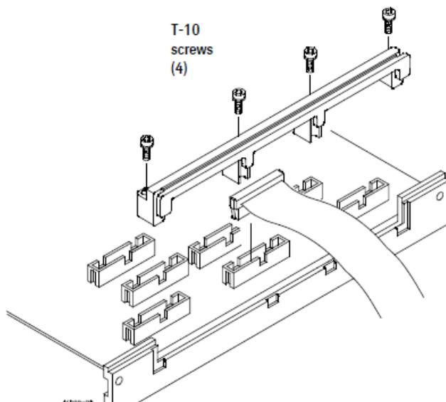
To remove and replace the pattern generator circuit board
