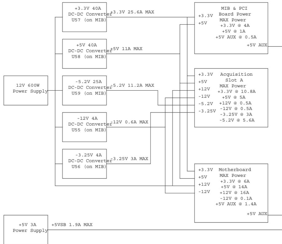
Power Supply Test Points on the 2-Slot, High-Power Frame
