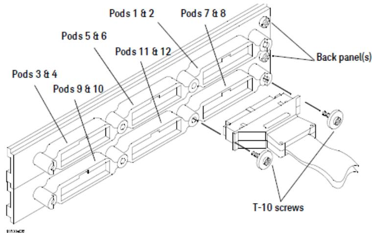
To remove and replace a measurement circuit board
