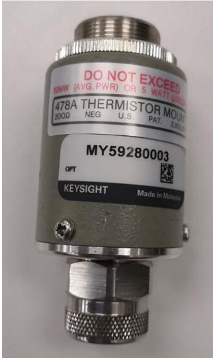
**Figure 1-1** Keysight Model 478A Thermistor Mount
