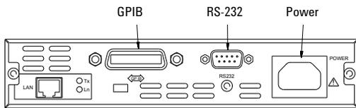
Connect GPIB and RS-232 cables. Plug AC Power cord into AC Power port on the E5810.
