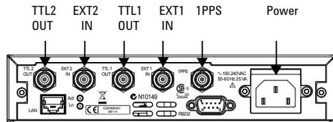
Connect BNC cables. Plug AC Power Cord into AC Power port and the E5818.
