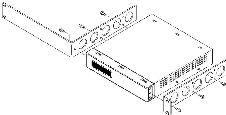
This rack mount is suitable for both E5810 and E5818 units.
