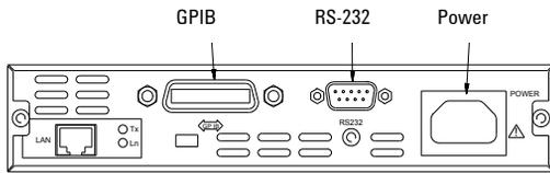
Connect GPIB and RS-232 cables. Plug AC Power cord into AC Power port on the E5810.
