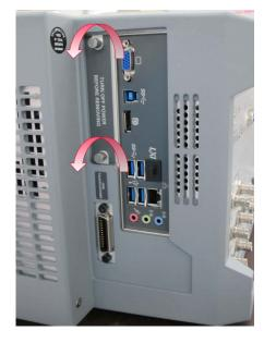
**Step 3.** Pull the housing to remove the solid-state drive.
