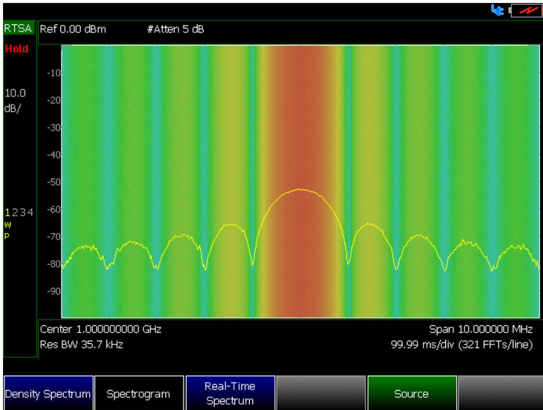
**Figure 6.** A signal captured using RTSA mode with gap-free results
