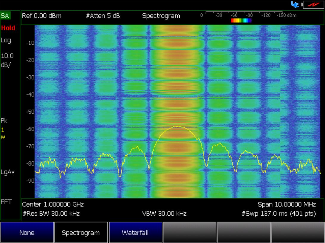
Figure 5. A signal captured using traditional spectrum analysis mode with dead time between updates
