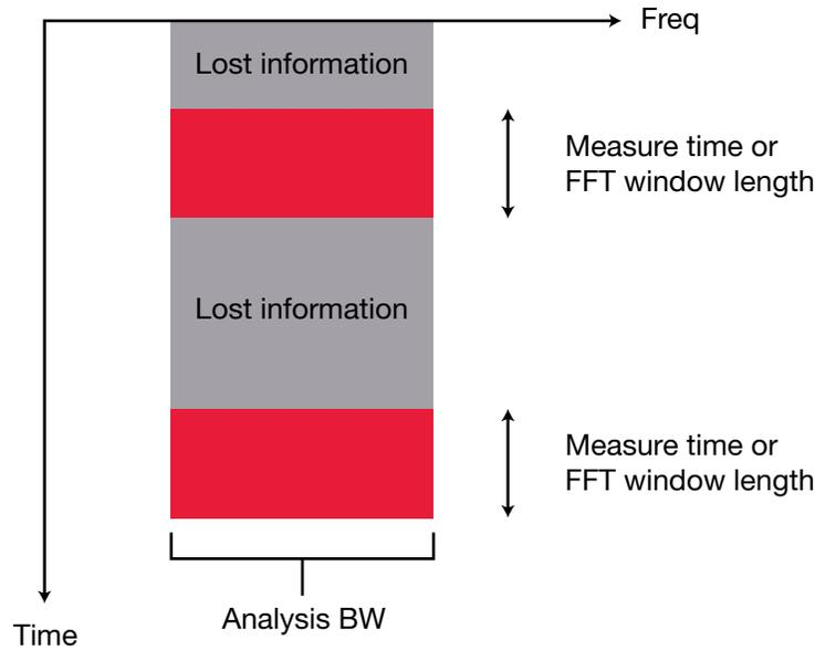
**Figure 4.** An FFT-based analyzer misses events that occur between time data sample blocks
