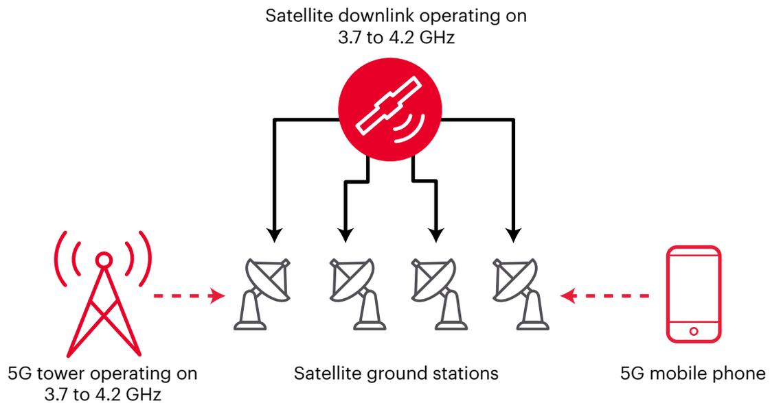
**Figure 2.** 5G radio tower and mobile phone interfering with satellite ground station communications
