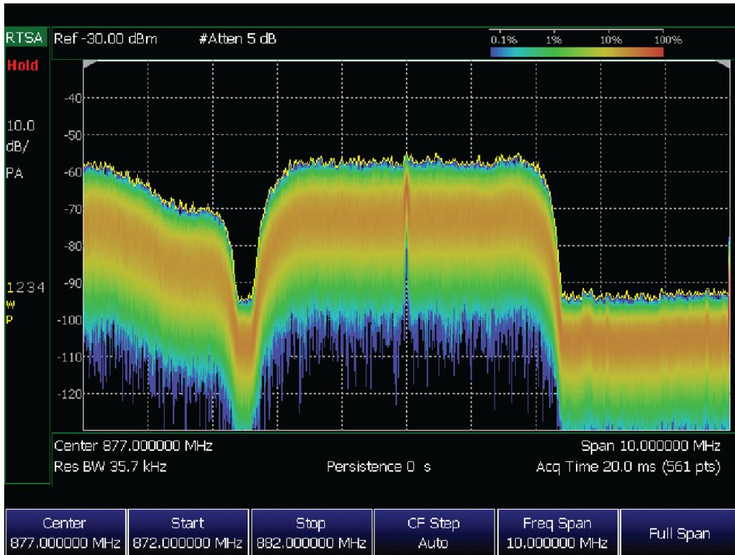
**Figure 8.** A signal captured using FieldFox's RTSA density display where the interfering signal is seen in the middle of the screen
