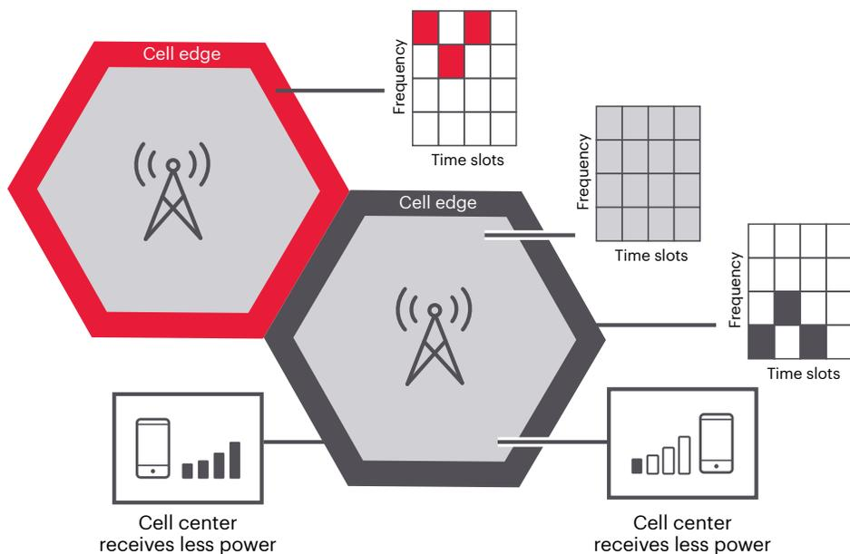
Figure 1. LTE power control and resource block allocation
