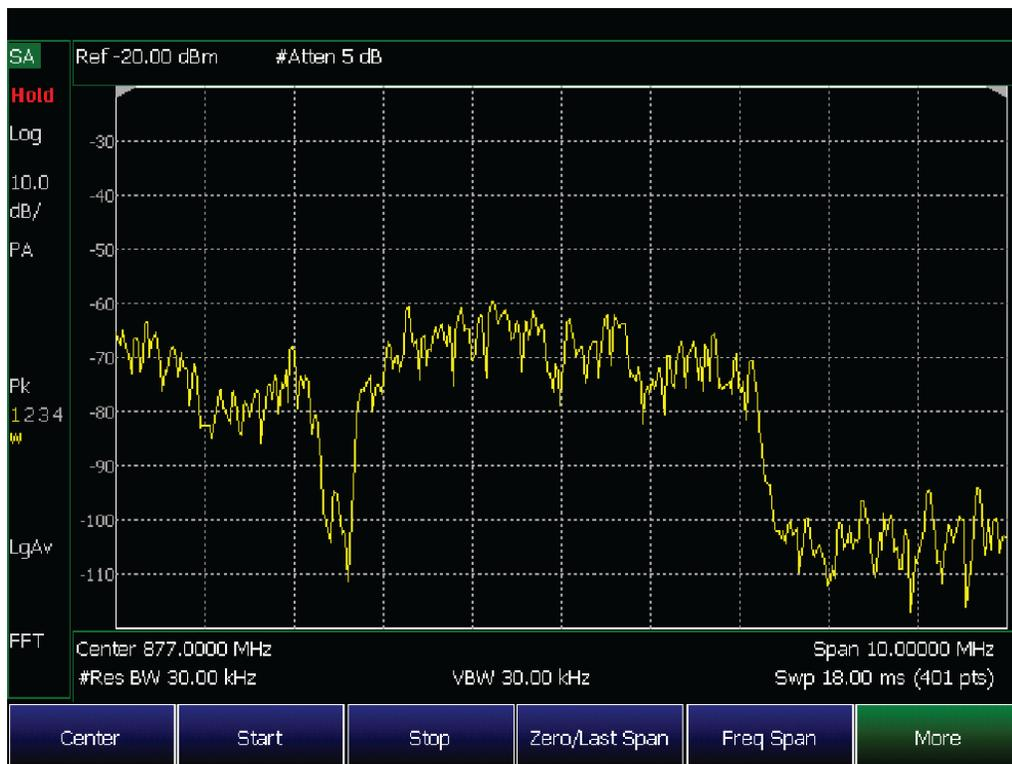
Figure 7. A signal captured using FieldFox’s traditional SA mode where the carrier signal masks the interfering signal
