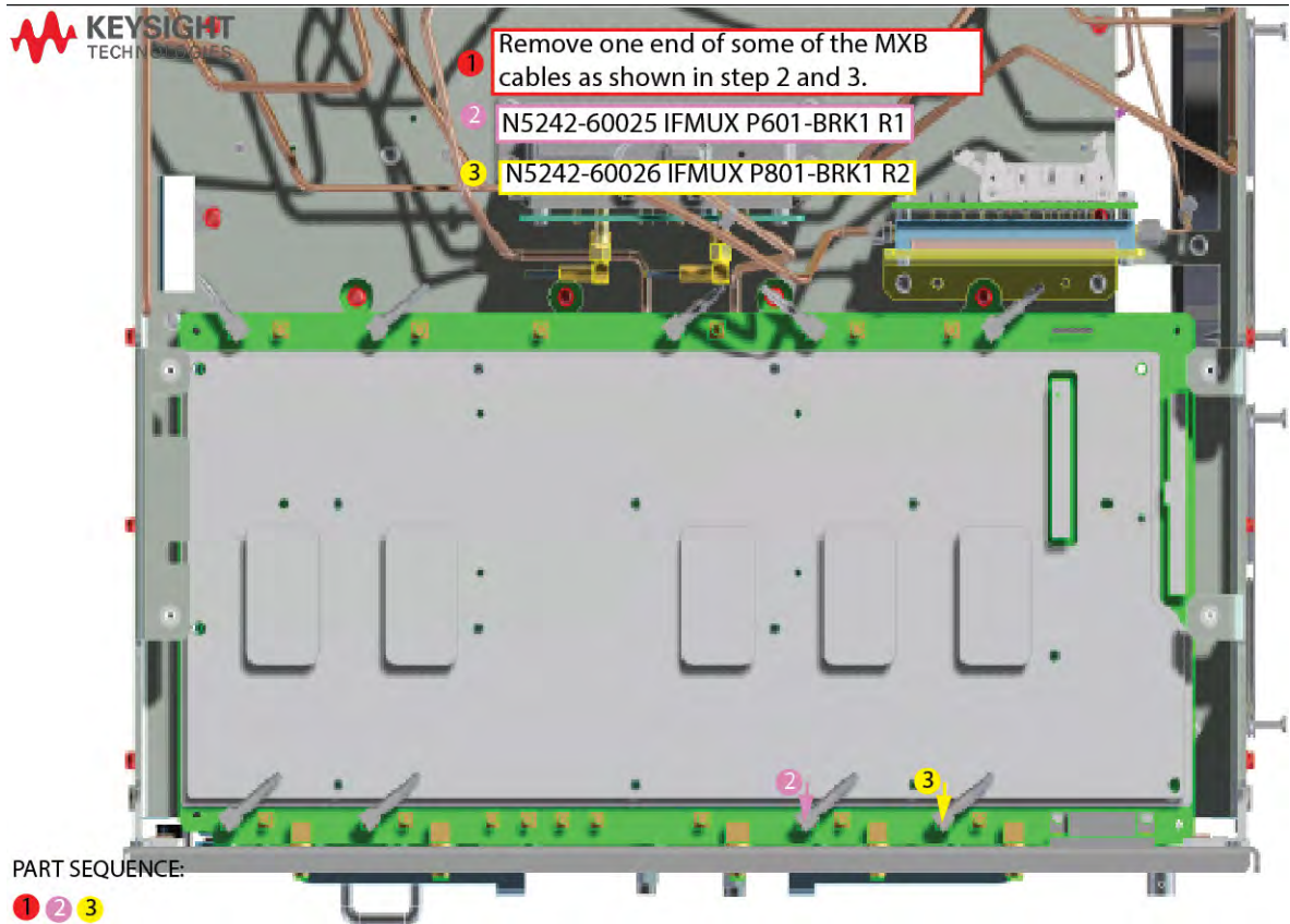
Figure 5 Remove the one end of the IF gray cables to the IF MUX board (N5242-60025 and N5242-60026)
