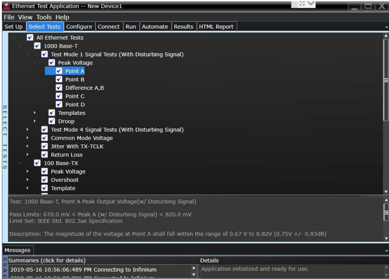
**Figure 2.** The Keysight automated test engine quickly guides you through selecting and configuring tests, setting up the connection, running the tests, and viewing the results. You can easily select individual tests or groups of tests with a mouse-click.
