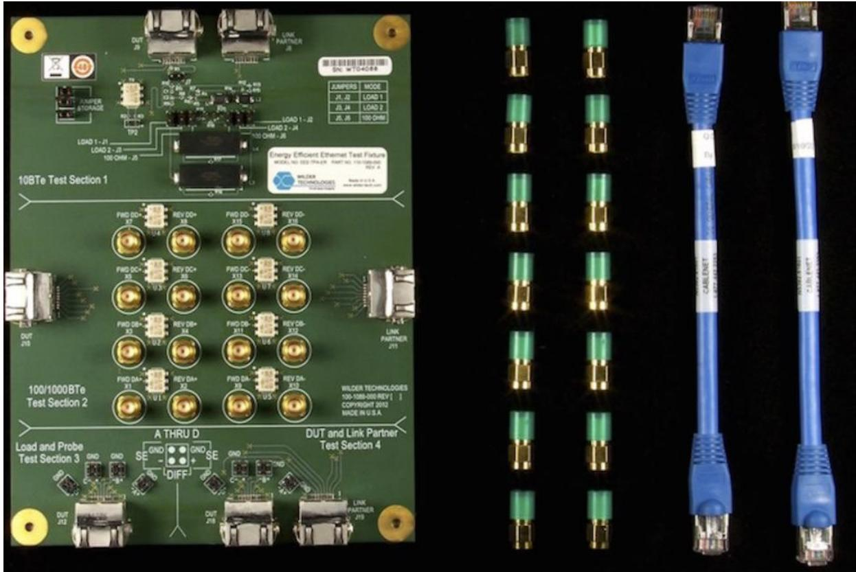
**Figure 9.** The EEE-TPA-ERK Wilder Technologies Energy Efficient Ethernet test fixture allows you to test to the 10BASE-T<sub>e</sub>, 100BASE-T<sub>Xe</sub> and 1000BASE-T<sub>e</sub> Energy Efficient Ethernet standards. Sold separately through Wilder-Technologies.
