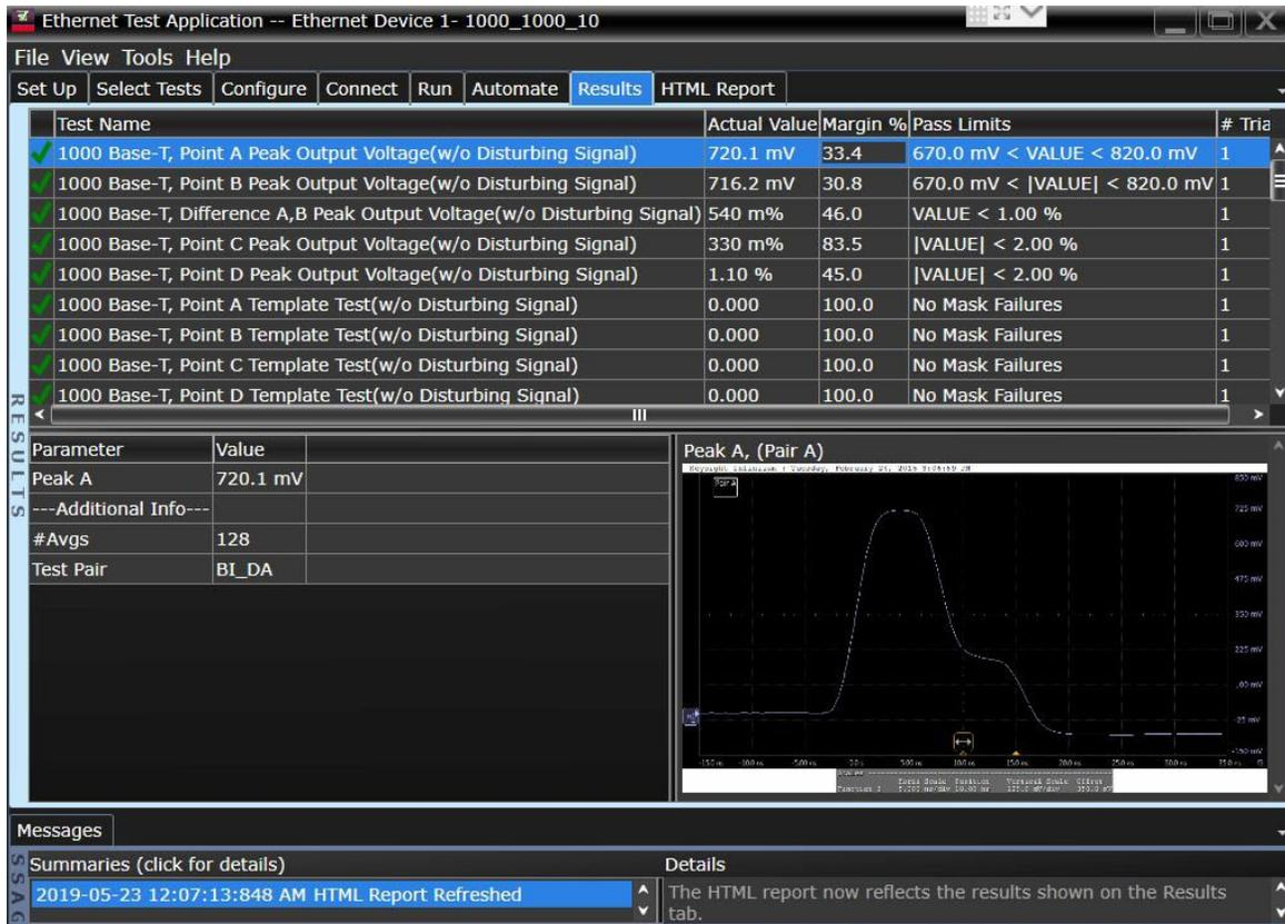
**Figure 5.** The D9010ETHC 10M/100M/1GBASE-T with Energy Efficient Ethernet compliance test application software results screen shows a summary of the tests performed, pass/fail status, and margin. Hyperlinks direct you to the more details of that test.
