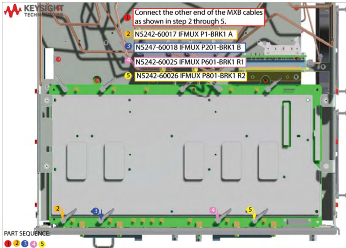
Figure 10 Reconnect the other end of the IF gray cables to the IF MUX board
