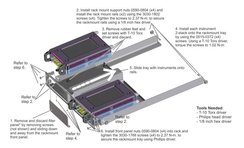
Installation of Two-High Rack Mount with Two Instruments \*Filler panel is only removed/discarded in a Two-unit installation.
