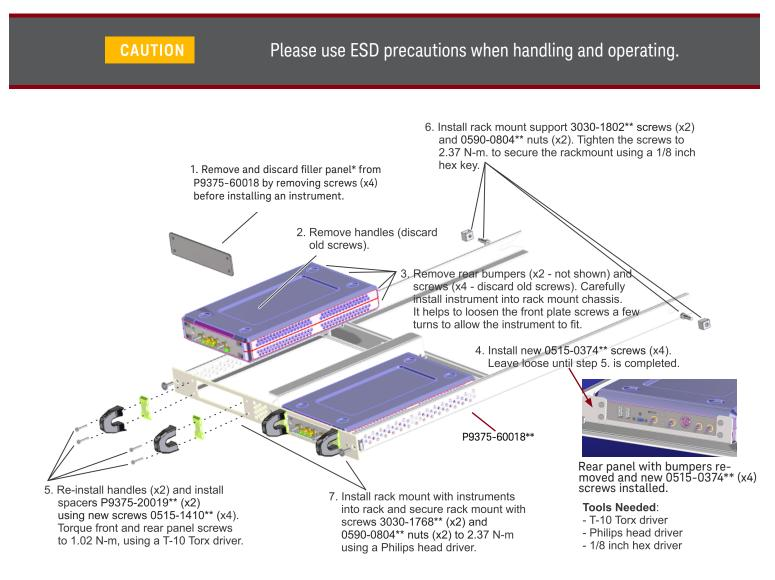
Installation of 1-High Rack Mount with Two Instruments \*Filler panel is only removed/discarded in a 2-unit installation. \*\*Lower level materials for P9375-60015
