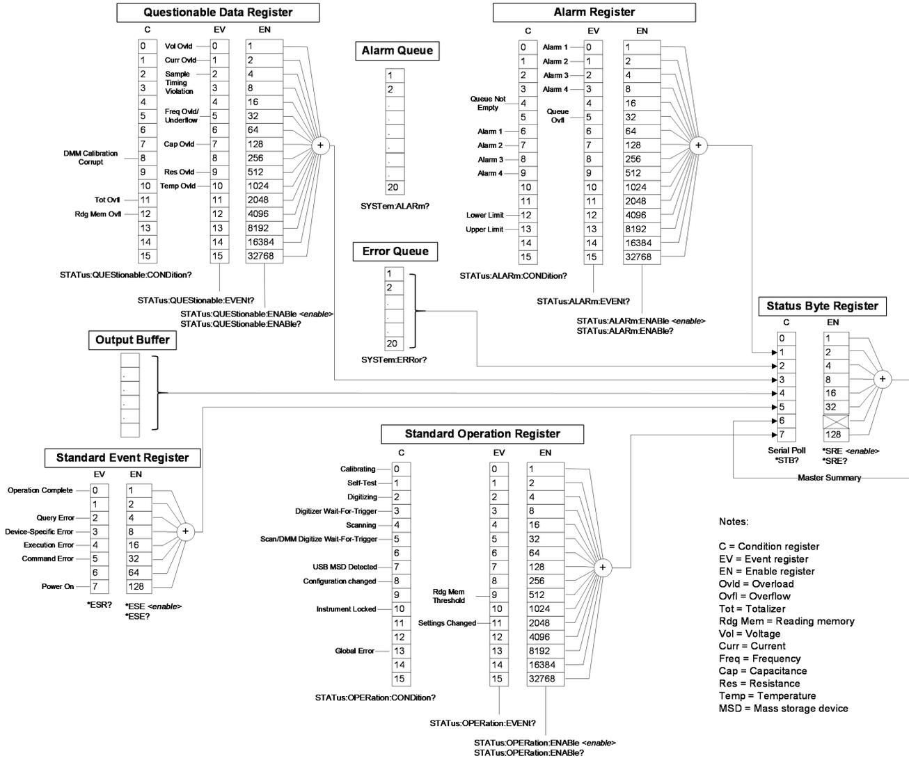
**Condition register (C)** - A condition register continuously monitors the state of the instrument. The bits in the condition register are updated in real time and the bits are not latched or buffered.
