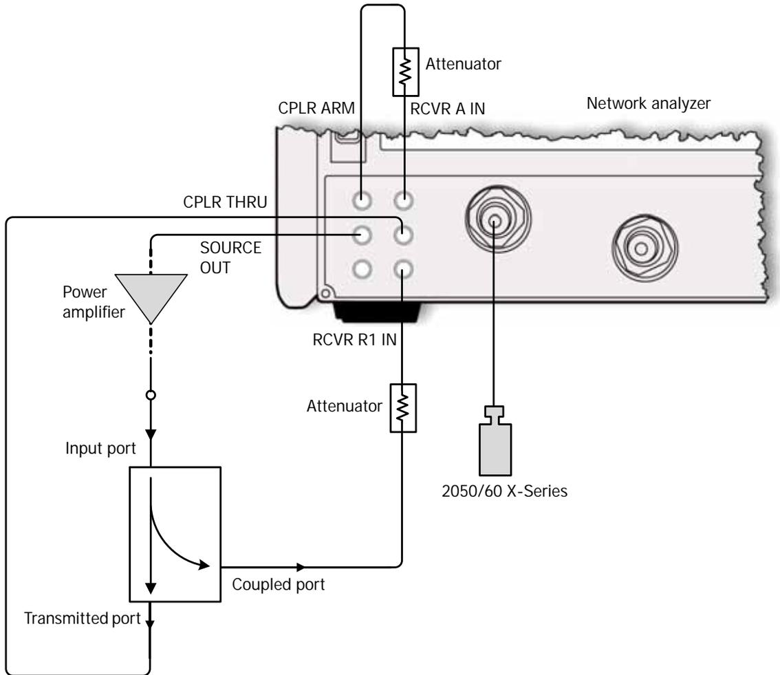
Figure 2-2 Equipment setup for high power S11 verification
