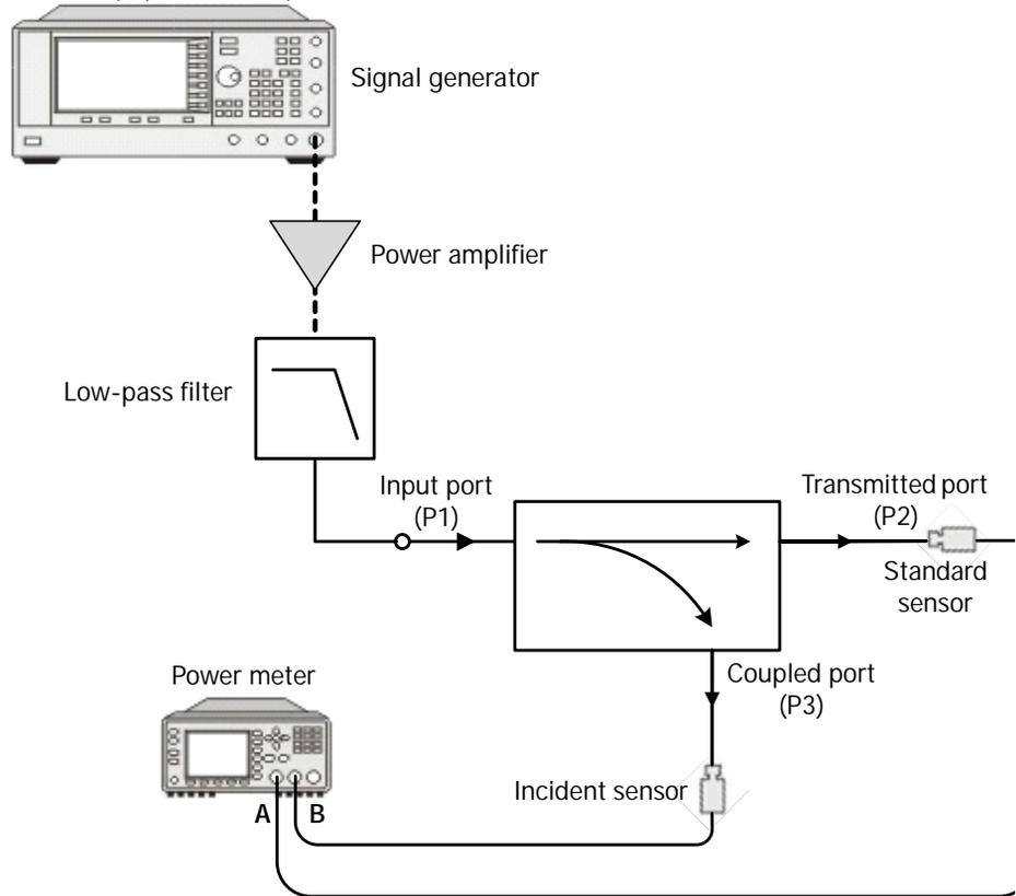
Figure 2-4 Equipment setup for high power verification
