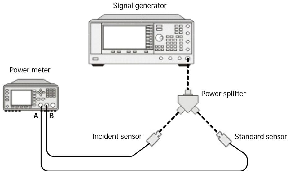
**Figure 2-3** Equipment setup for low power verification
