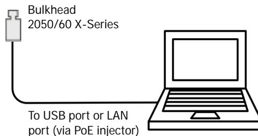
**Figure 2-5** Equipment setup for zero set verification
