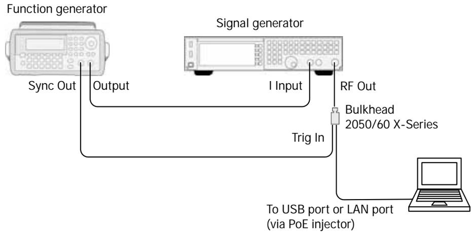
**Figure 2-6** Equipment setup for rise time verification
