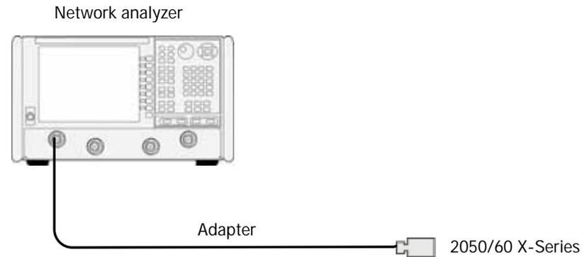
**Figure 2-1** Equipment setup for low power S11 verification
