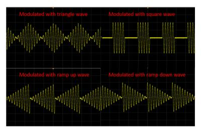
Figure 14. Various carrier signals used for waveform modulations (other than sine wave)
