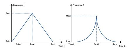
Figure 9. Frequency sweeps over time for linear and logarithmic spacings.
