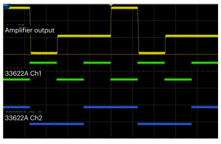
**Figure 8.** Two phased synchronized signals from the function generator and the resultant output signal from the differential amplifier
