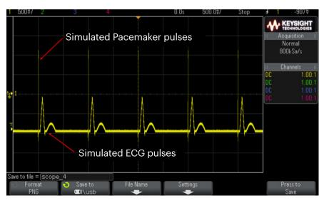
Figure 2. Resultant waveform by combining the above two waveforms
