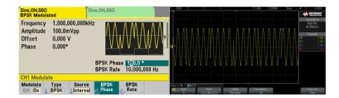
Figure 16. Simple BPSK modulation setup and output shown on oscilloscope
