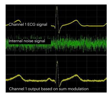
**Figure 4.** Combination of an ECG signal and a noise signal using the sum modulation capability of Keysight's 33622A function generator
