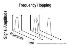
**Figure 12.** Graph shows user-defined radio frequency hopping over time
