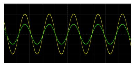
Figure 6. Two signals that are amplitude and phase coupled together
