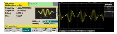
Figure 13. Simple amplitude modulation setup and output shown on oscilloscope
