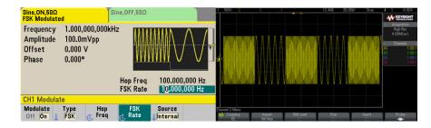
Figure 15. Simple FSK modulation setup and output shown on oscilloscope
