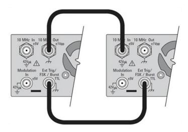
**Figure 18.** Example of a Keysight 33600A function generator's rear wire configurations on time-base and external trigger synchronization between two function generators
