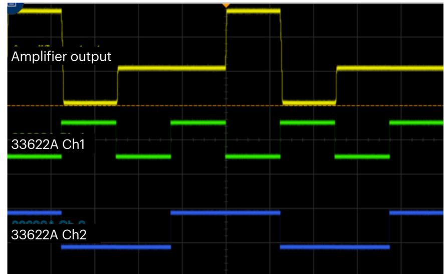
Figure 8. Two phased synchronized signals from the function generator and the resultant output signal from the differential amplifier
