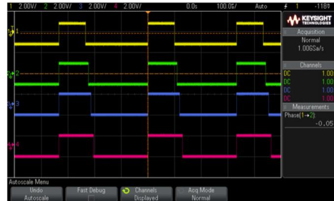
Figure 17. Time-synchronized, multi-channel outputs
