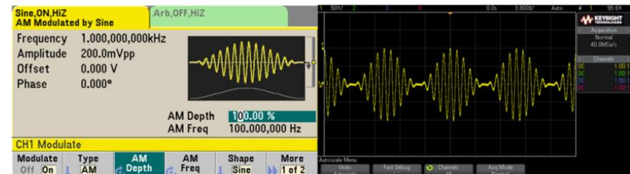
Figure 13. Simple amplitude modulation setup and output shown on oscilloscope
