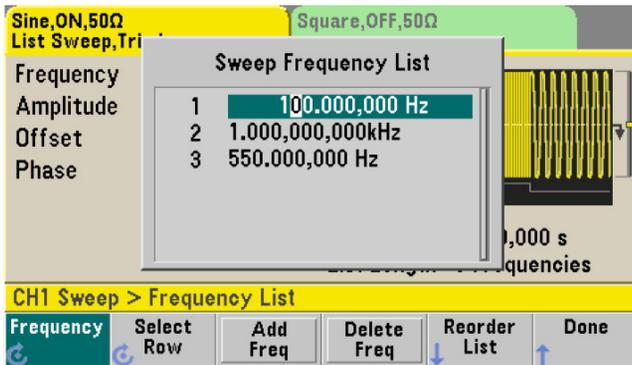
Figure 11. Sweep frequency list can simulate radio frequency hopping
