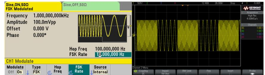
Figure 15. Simple FSK modulation setup and output shown on oscilloscope
