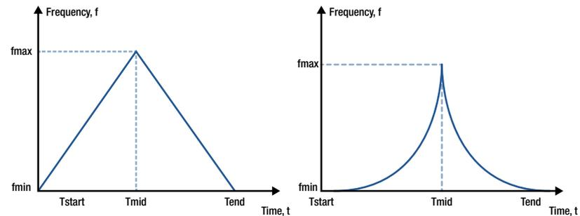
Figure 9. Frequency sweeps over time for linear and logarithmic spacings.
