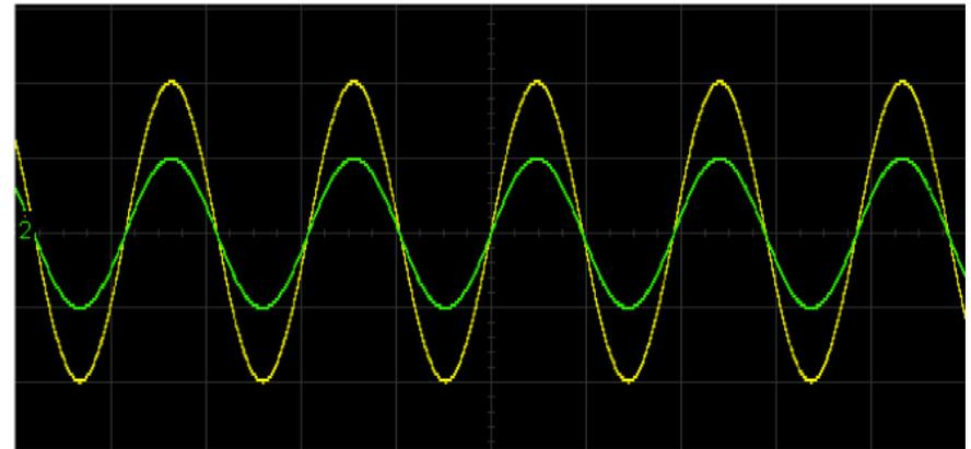
Figure 6. Two signals that are amplitude and phase coupled together
