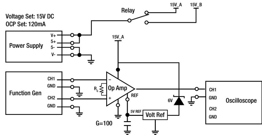
Figure 7. A diagram for setting up instruments to test a differential amplifier
