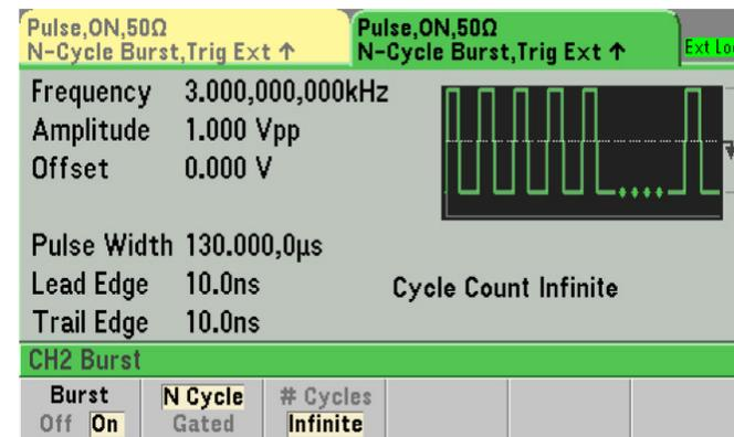
Figure 20. Burst mode setup menu on function generator
