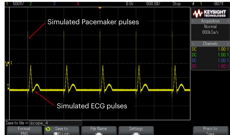
Figure 2. Resultant waveform by combining the above two waveforms
