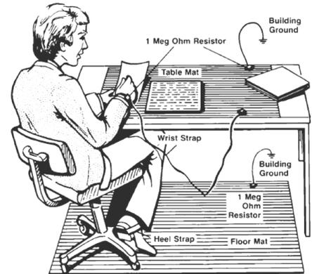
Both types, when used together, provide a significant level of ESD protection. Of the two, only the table-mat and wrist-strap combination provides adequate ESD protection when used alone. To ensure user safety, the static-safe accessories must provide at least 1 M $\Omega$  of isolation from ground.
