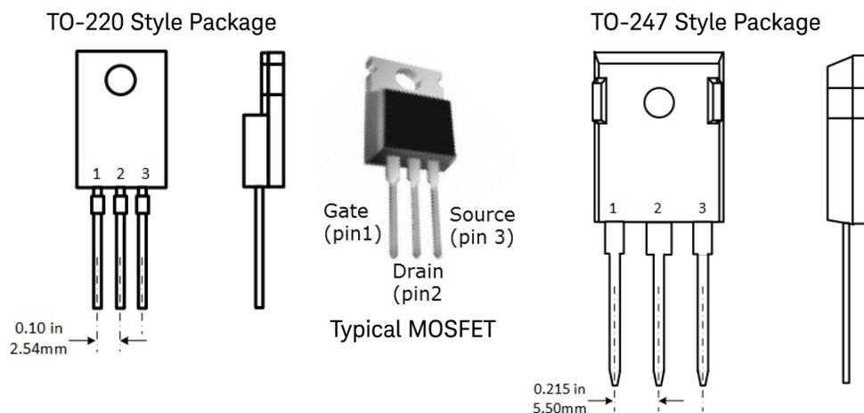
**Figure 6** Typical TO-220 Device and TO-247 Device Packaging
