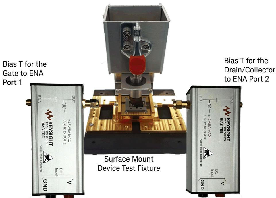
**Figure 3** PD1000A Bias T Networks with PD1000A SMD Test Fixture
