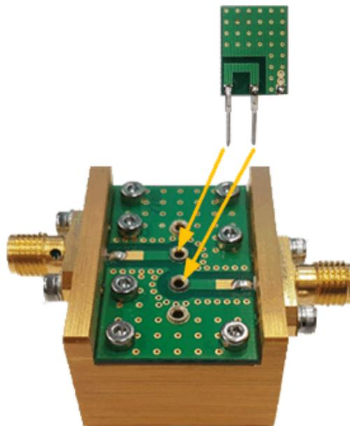
**Figure 15** Inserting the **THROUGH** Standard into the Test Fixture
