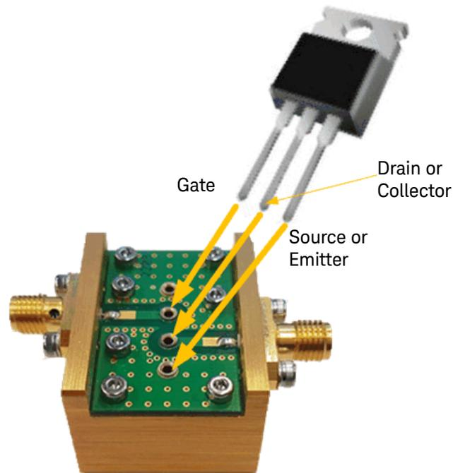
**Figure 7** Inserting TO- Style Devices into the TO-220/TO-247 Test Fixtures
