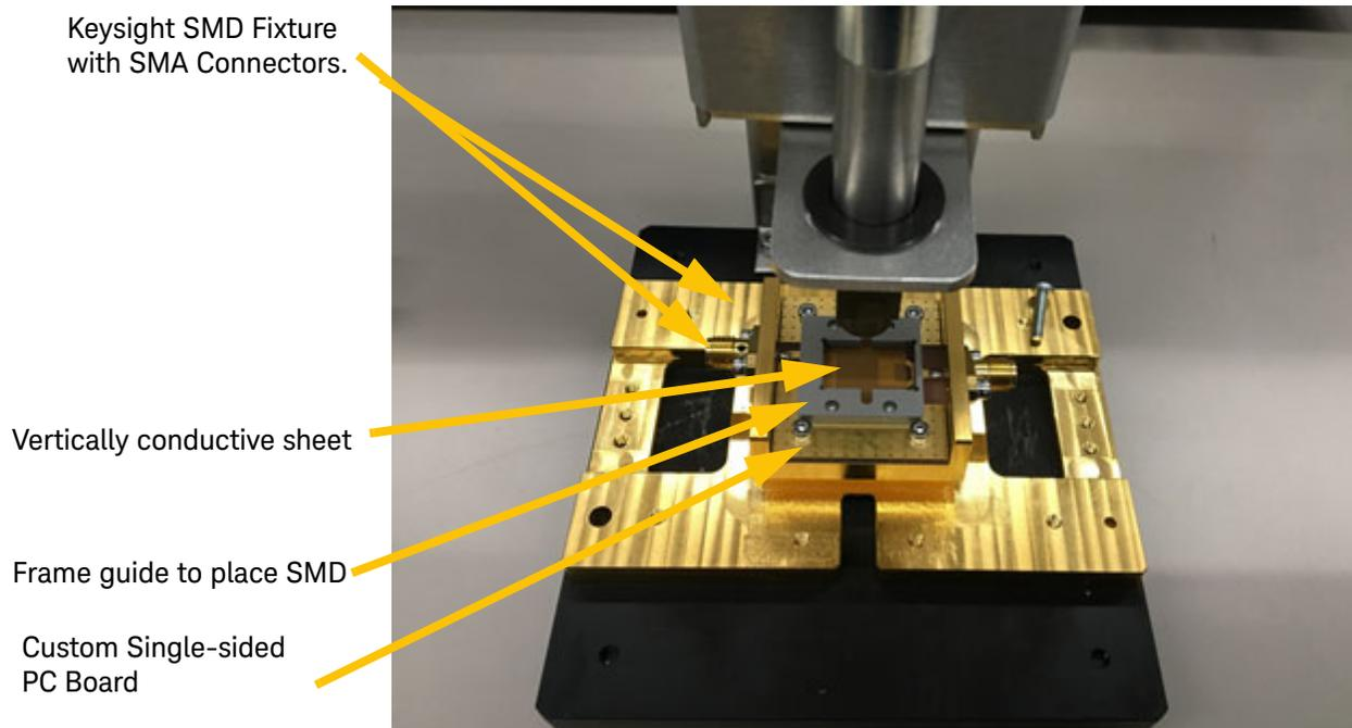
**Figure 23** Assembling the SMD Test Fixture
