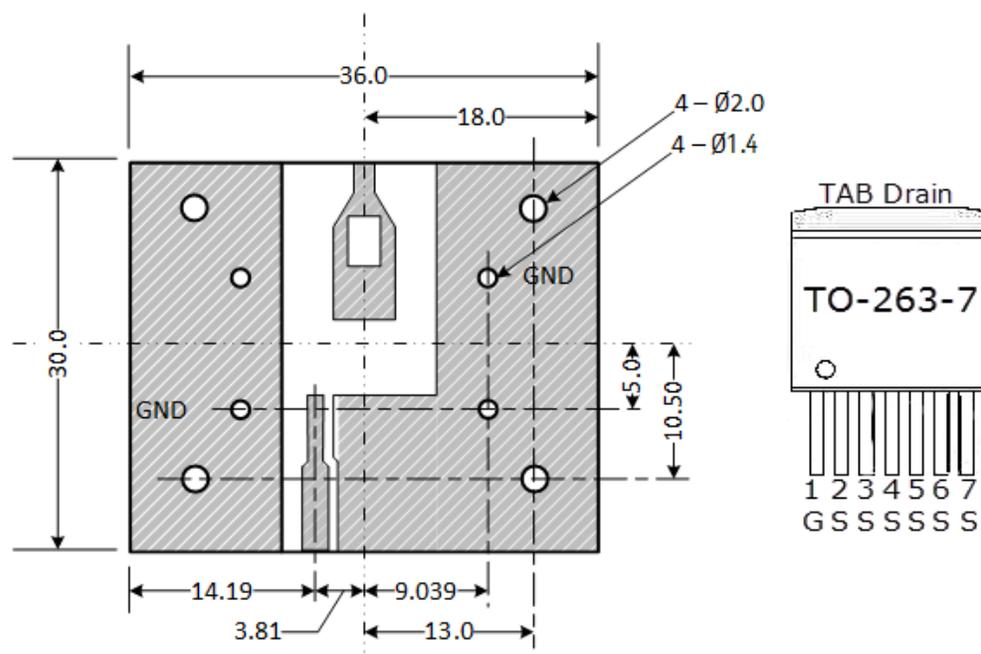
**Figure 18** PD1000A SMD Test Fixture PC Board Guidelines. All dimensions in mm.
