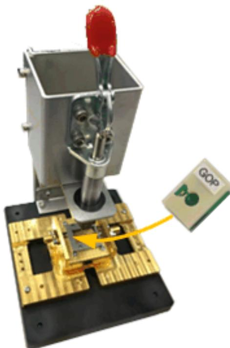
**Figure 16** Placing an **OPEN**, **SHORT**, or **LOAD** Standard into the SMD Test Fixture
