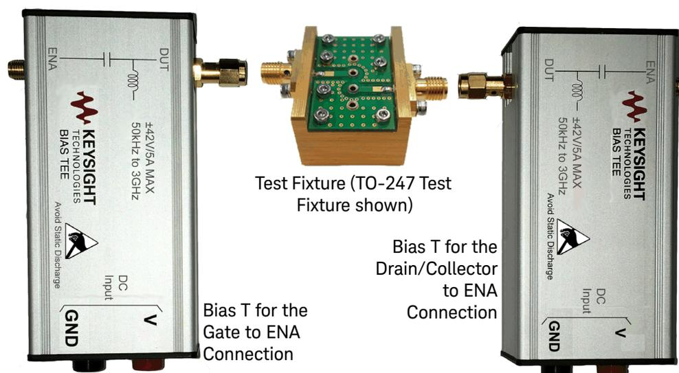
**Figure 2** PD1000A Bias T Networks with TO-220 and TO-247 Test Fixture
