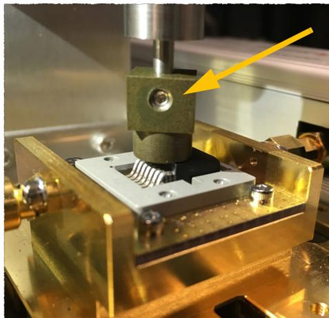
**Figure 24** Allen Screw to Adjust the Height of the Push Rod
