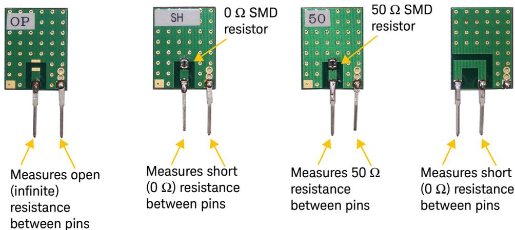
**Figure 26** Measuring the DC Resistance of the TO-220/TO-247 Cal Standards
