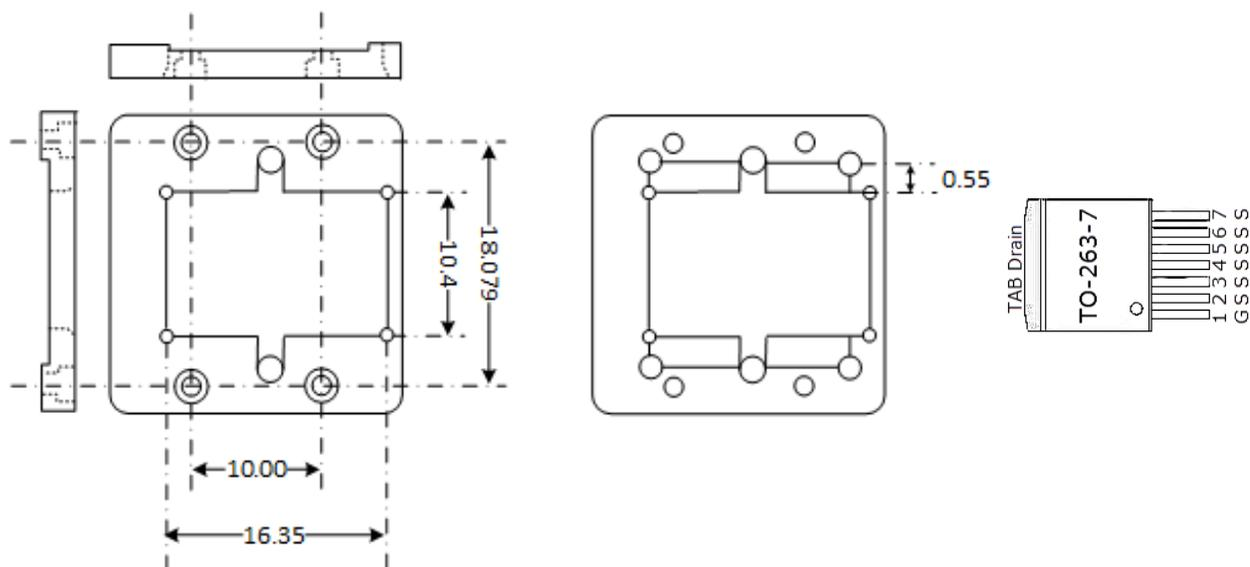
**Figure 20** PD1000A SMD Frame Guide Outside Dimensions. Inside dimensions are for a TO-263-7 package. TO-263-7 shown for orientation purposes. All dimensions in mm.
