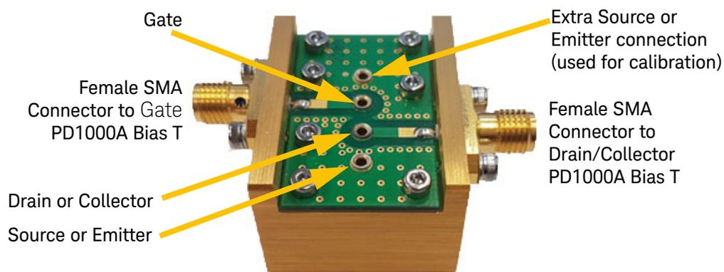
**Figure 5** Keysight PD1000A TO-247 and TO-220 Test Fixture
