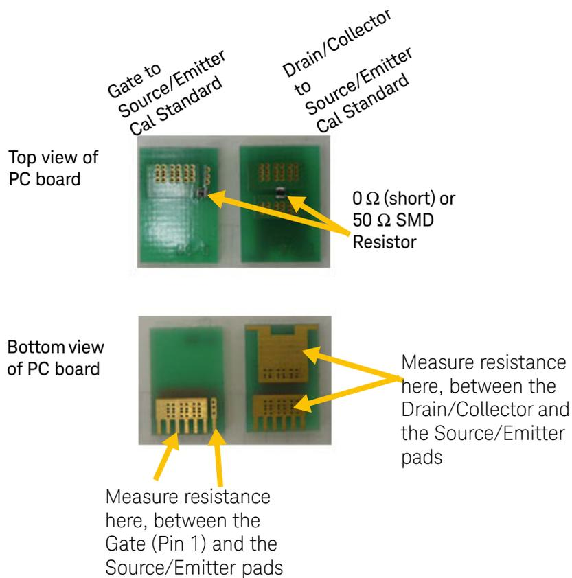
**Figure 27** Measuring the DC Resistance of the SMD Calibration Standards
