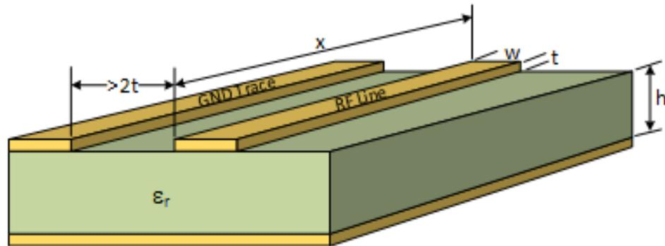
**Figure 19** Microstrip Line Example for 50 Ω Impedance
