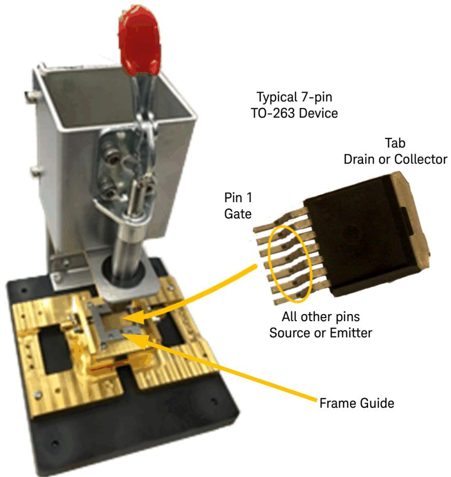
**Figure 9** Inserting Surface Mount Devices into the SMD Test Fixture
