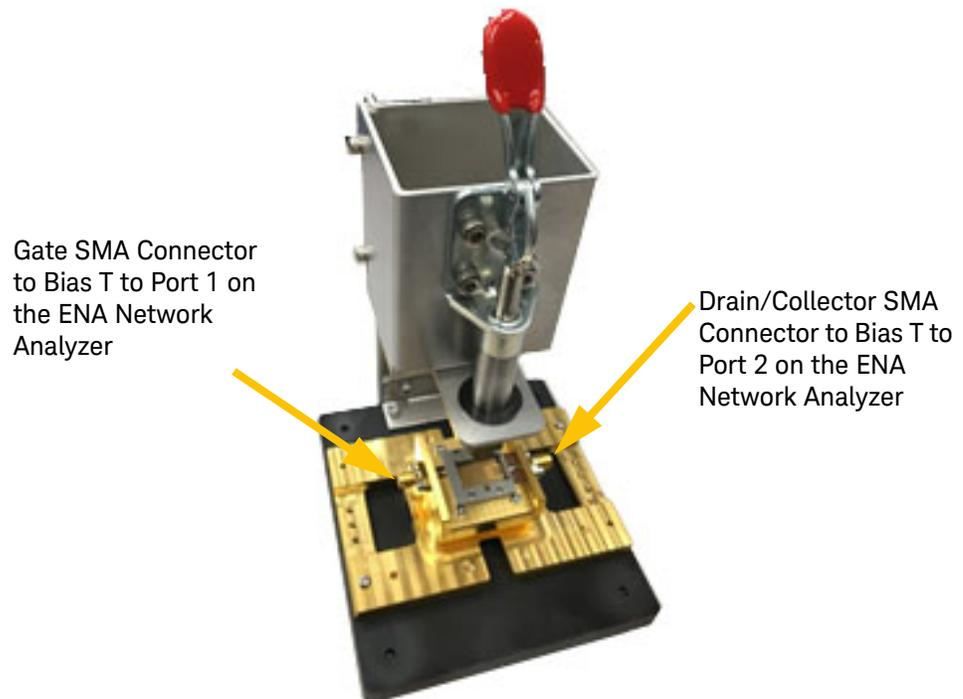
**Figure 8** Keysight PD1000A Surface Mount Device Test Fixture
