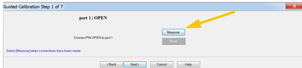
10 Insert the Port 1 **OPEN** Cal Standard into the test fixture. The **OPEN** Cal Standard goes between the Gate and Drain/Collector. Click **Measure**.
