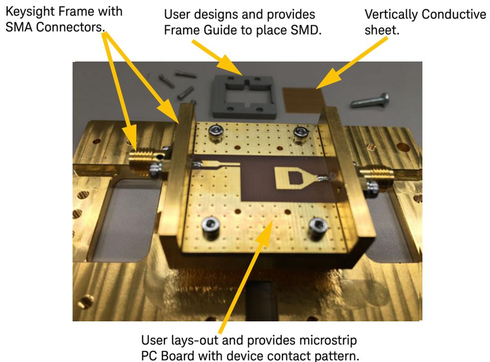
**Figure 17** PD1000A SMD Test Fixture Components
