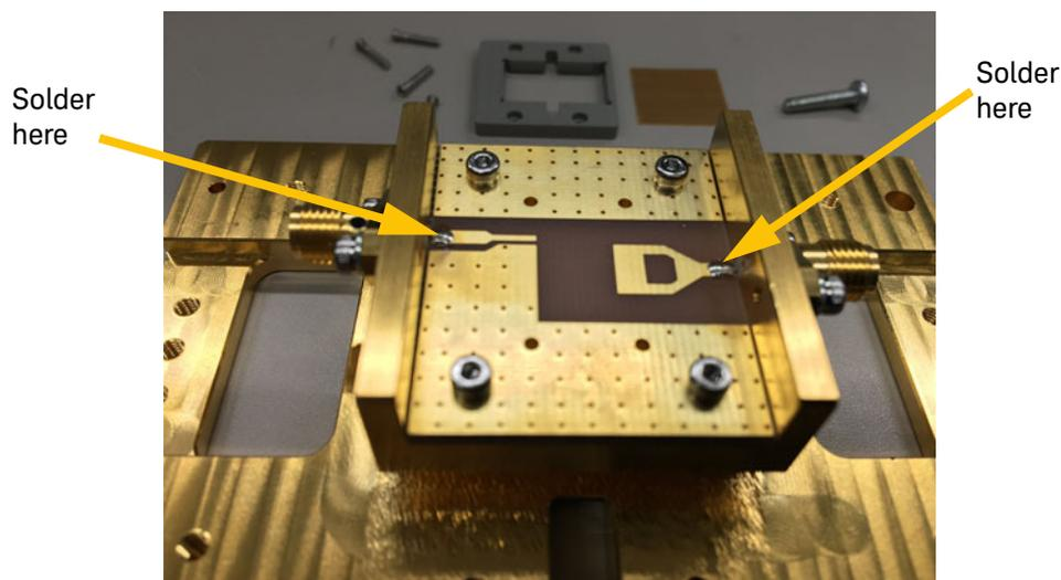
**Figure 22** Solder the PC Board Pads to the SMA Connector Pins
