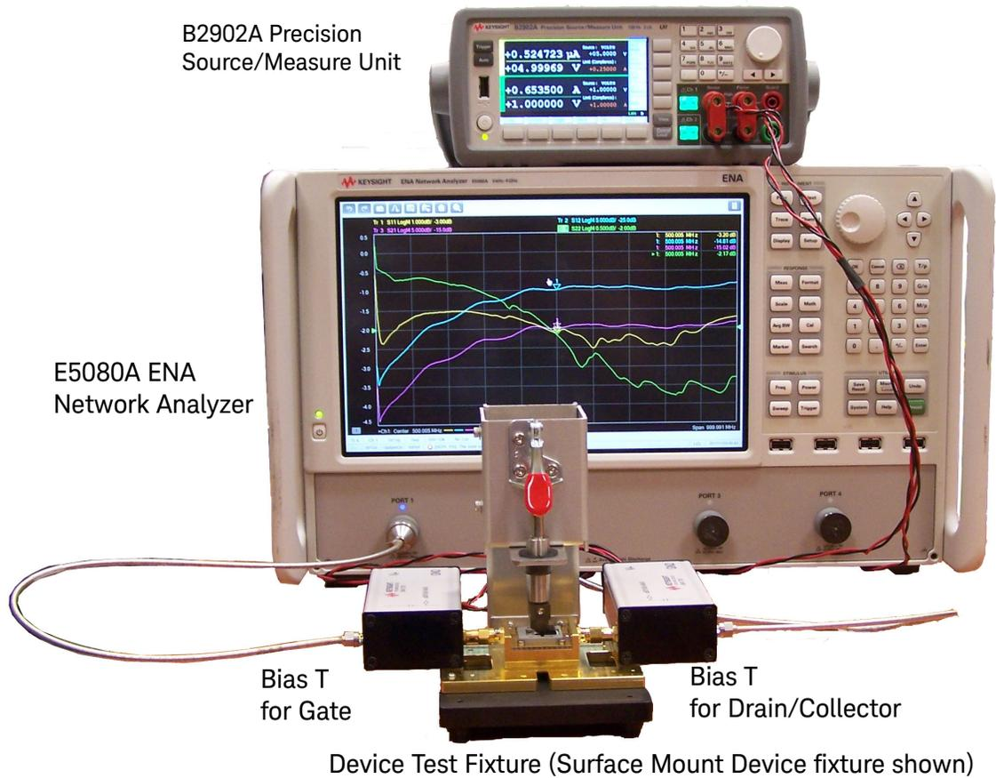
**Figure 12** Calibration Setup for the PD1000A SMD Test Fixture. Setup for the TO-220/TO-247 Fixtures is similar.
