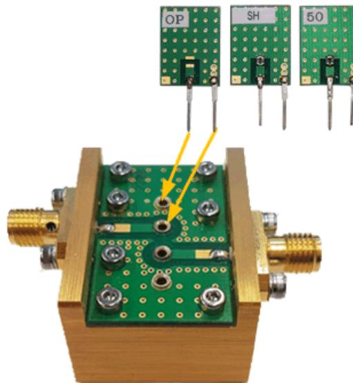
**Figure 13** Inserting the Input **OPEN**, **SHORT**, **LOAD** Standards into the Test Fixture
