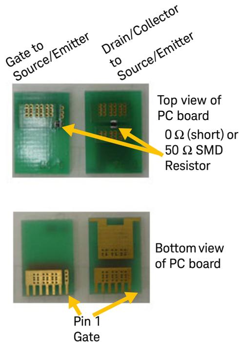
Example Calibration Standards for the “Gate to Source/Emitter” and the “Drain/Collector to Source Emitter”. The traces on the bottom of the PC Board must match the pin-out of the DUT. The 0 Ω SMD resistor (short) or 50 Ω SMD resistor must be placed on the top of the PC Board.
