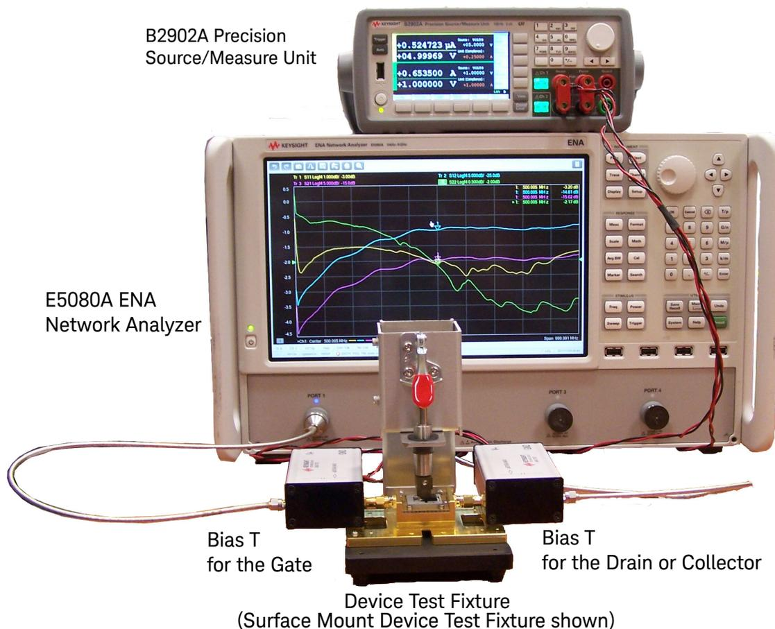
**Figure 1** General Test Setup for the PD1000A S-Parameter Test System
