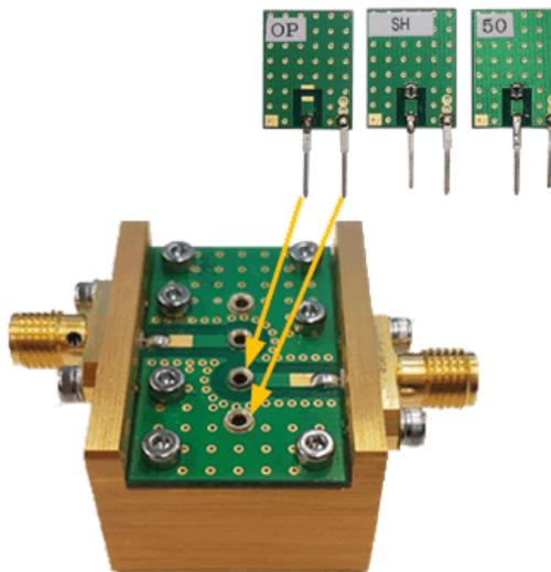
**Figure 14** Inserting Output **OPEN**, **LOAD**, or **Short** Standards into the Test Fixture
