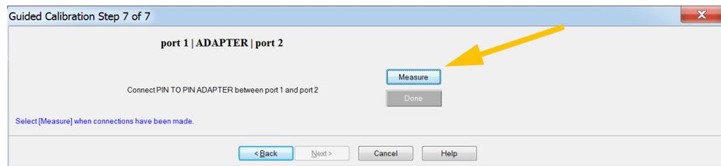
**16** Insert the **THROUGH** Calibration Standard into the Test Fixture. Click **Measure**.
