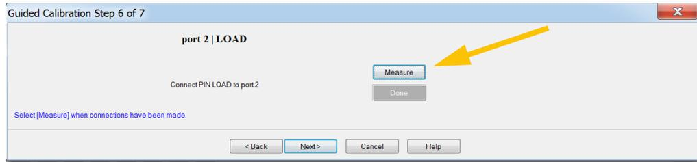
**15** Insert the Port 2 **50 Ω LOAD** Cal Standard into the test fixture. The **50 Ω LOAD** Cal Standard goes between the Gate and Drain/Collector. Click **Measure**.
