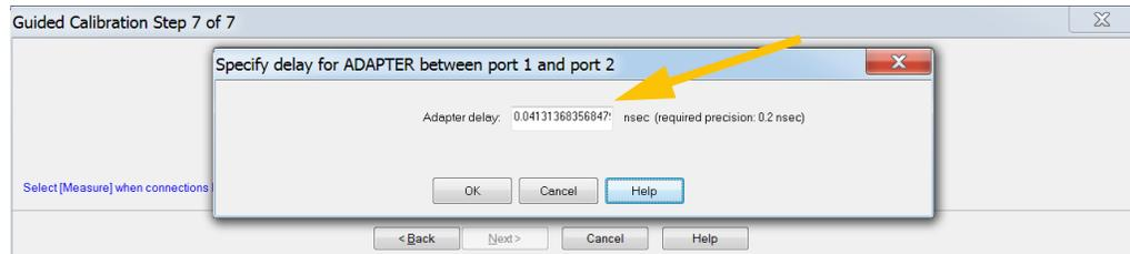
**17** In this screen, the display shows the calculated delay through the **THROUGH** Cal Standard. Ensure that the displayed value is less than 0.2 nS. Click **OK**.
