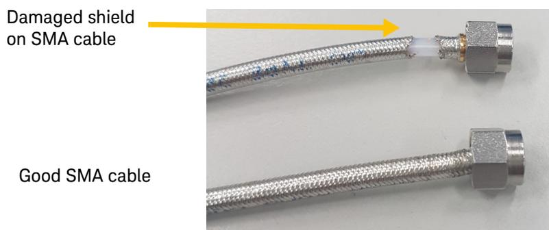
**Figure 25** Damaged SMA Cable
