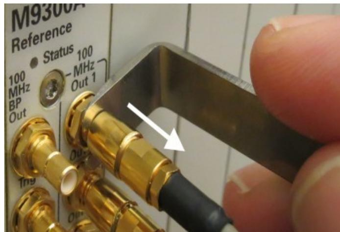
To avoid damage to the cables or connectors, pull the cable straight away from the connector. Do not use the tool as a pry bar.
