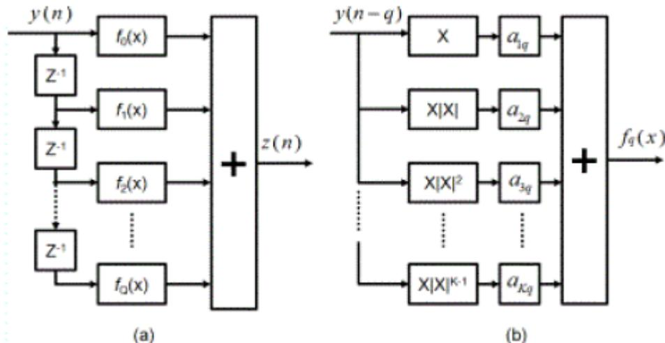
The structure of Volterra series is shown below.
