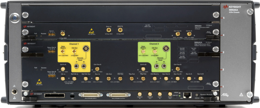
Figure 32 Installed M8045A and M8046A module
