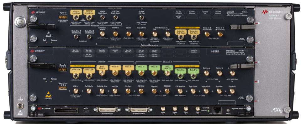
Figure 3 M8020A configuration for 32 Gb/s BERT
