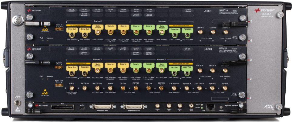
Figure 2 M8020A configuration for 16 Gb/s BERT for up to 4 channels
