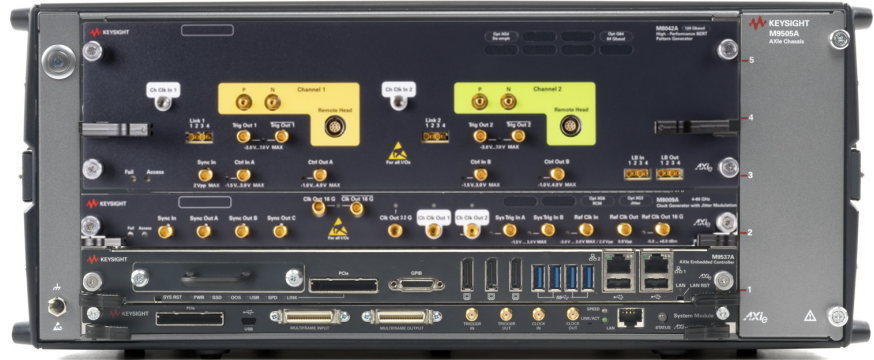
Figure 40 Installed M8042A module in slots 3 through 5
