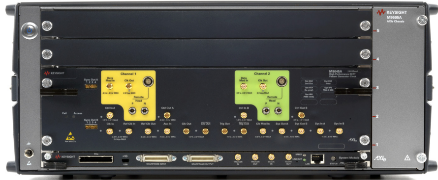
Figure 29 Installed M8045A module in slots 1 through 3
