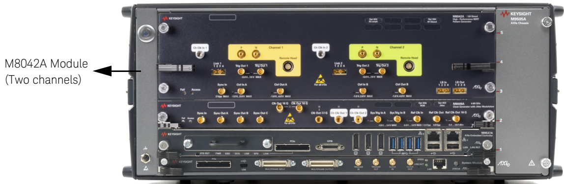
Figure 9 M8009A, M8042A (two channels) configuration
