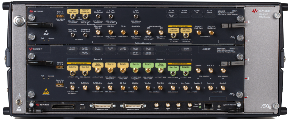
Figure 22 Installed M8041A and M8062A module
