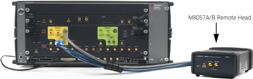
Figure 7 M8045A, M8046A and M8057A/B configuration
