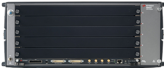
Figure 13 M9505A 5-slot chassis
