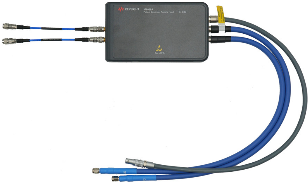
Figure 47 Connecting 150 mm cables to M8050A remote head
