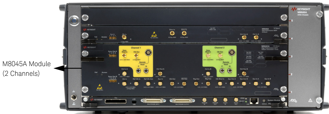
Figure 5 M8045A configuration for 2 channels
