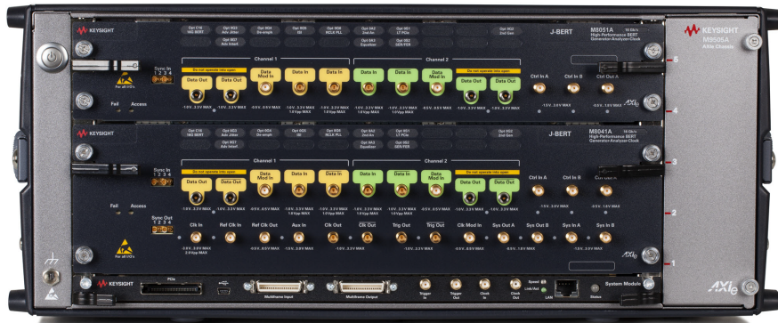
Figure 17 Installed M8041A and M8051A module
