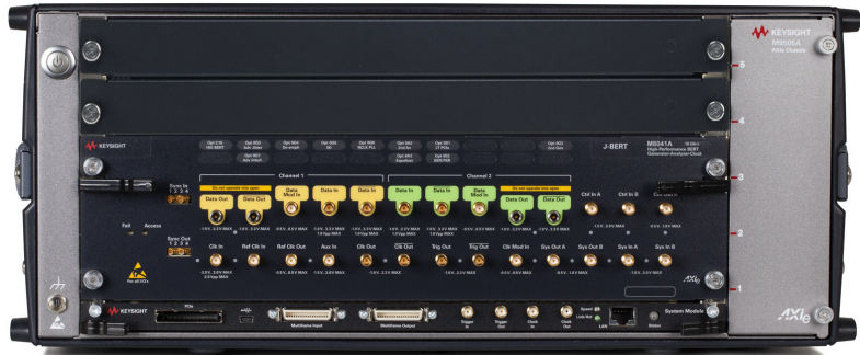
Figure 14 Installed M8041A module in slots 1 through 3
