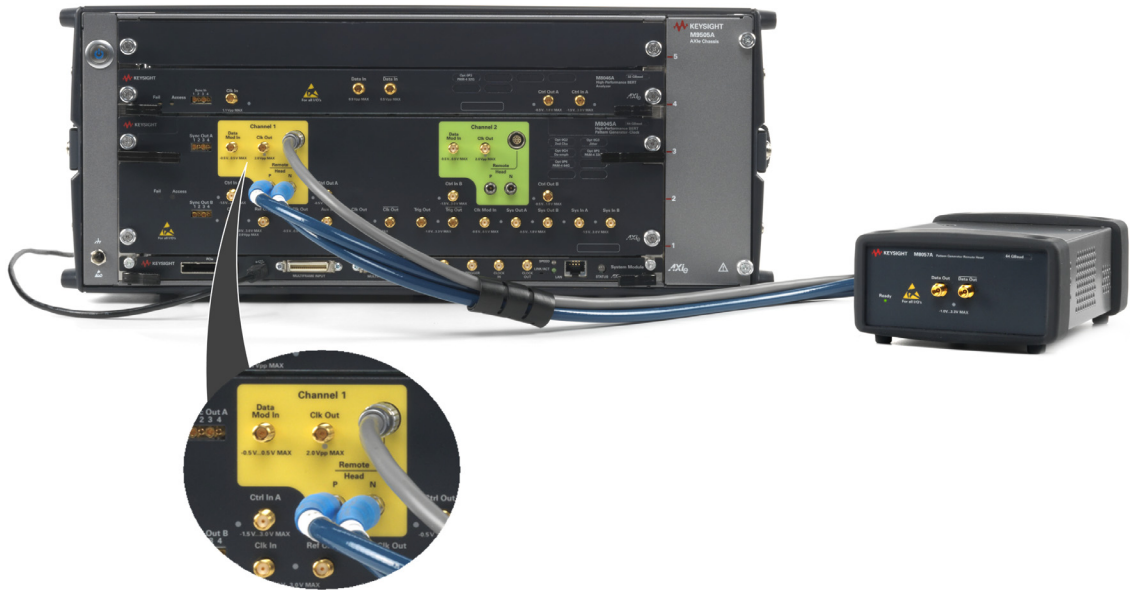
Figure 35 Installing M8045A, M8046A modules and M8057A/B remote head
