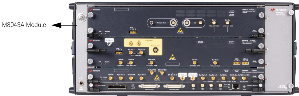
Figure 10 M8009A, M8042A (one channel) and M8043A configuration
