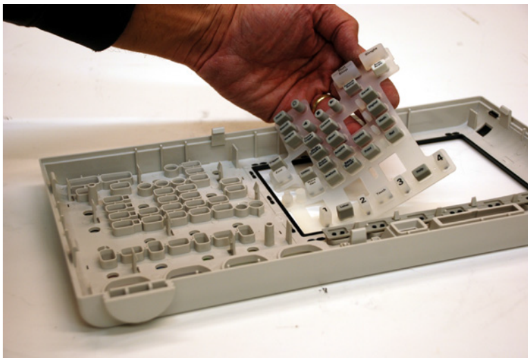
Figure 53 Remove the keyboard keypad from the bezel
