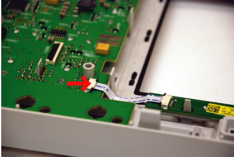
Figure 49 Disconnect the softkey board cable
