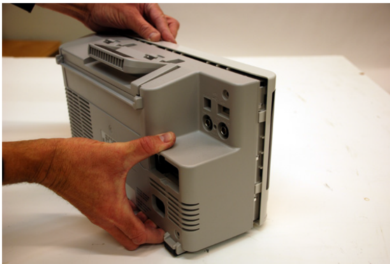
Figure 23 Removing bucket assembly
