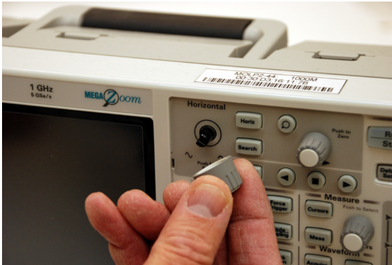
Figure 21 Removing the front panel knobs
