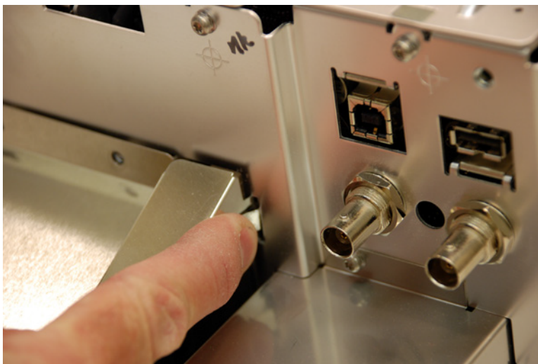
Figure 25 Unclipping the power supply shield right side
