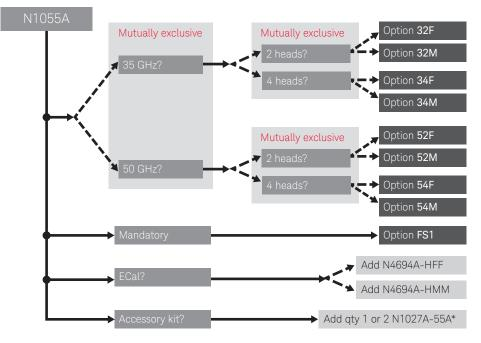
\* Each N1027A-54A accessory kit supports two differential channels (four heads).
