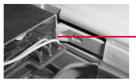
Make sure that shield is locked in place behind this tab.
