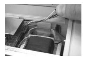
7 Insert the DMM input cable into the backplane connector.
