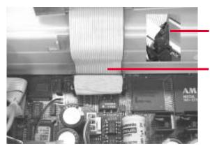
Snap Locking Clips over the top of the connector to secure the Ribbon Cable.
