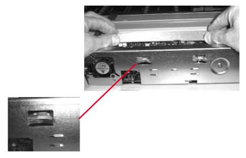
**5** Lock the internal DMM circuit board in place.
