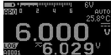
The maximum number of readings that can be stored for the interval log is 3000 entries. When all entries are occupied, **A : FULL** will be shown when you press and hold
