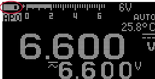
Replace the batteries as soon as possible when the low battery indicator (
