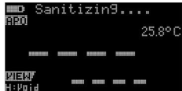
Prior to sanitizing the log memories, ensure that all manual (**H**), interval (**A**), or event (**E**) records have been cleared (see [step c](#)). When all entries are cleared (**H : Void**, **A : Void**, and **E : Void**), press and hold
