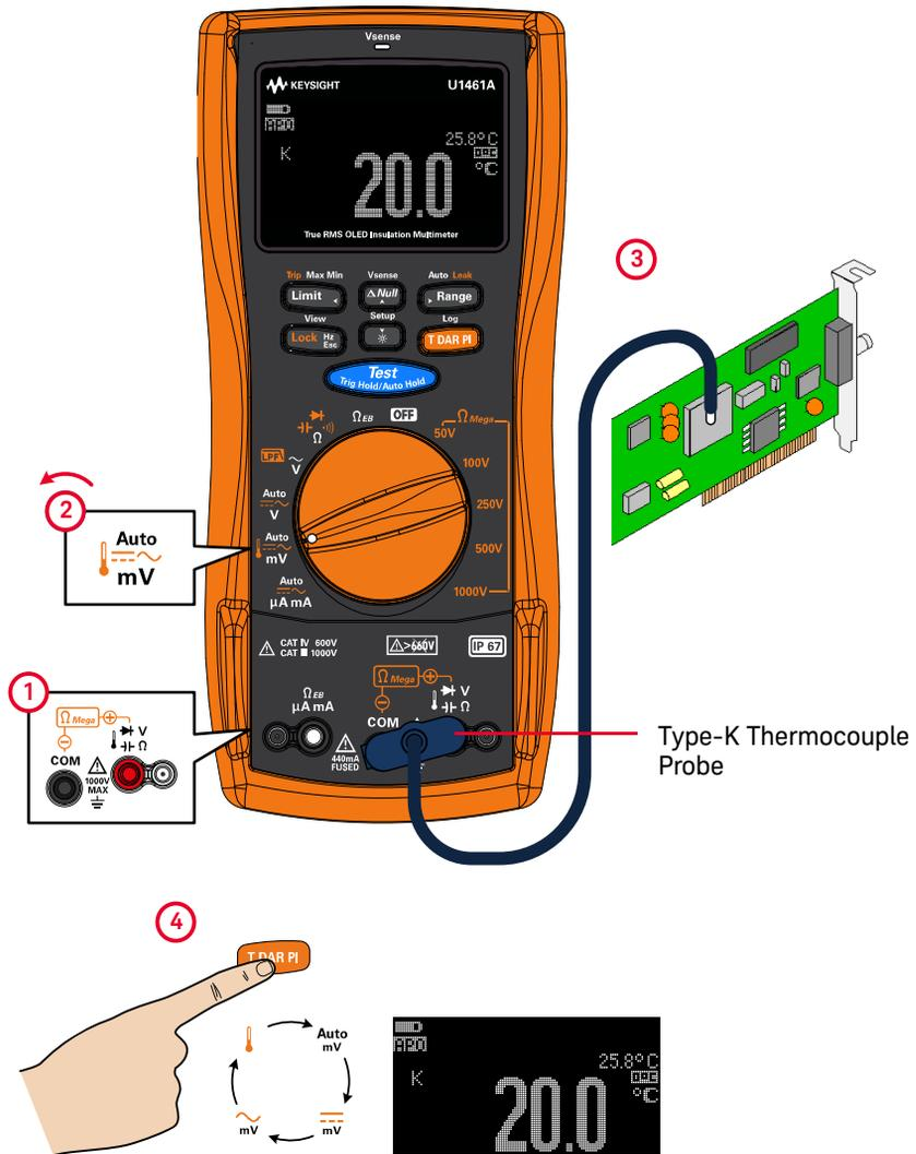
Figure 2-22 Surface temperature measurement example
