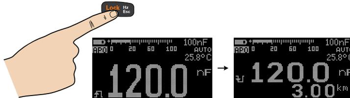
The default cable length scale is 1 km per 40 nF (km/C). To change this value, see [“Changing the cable length scale”](#) on page 145.
