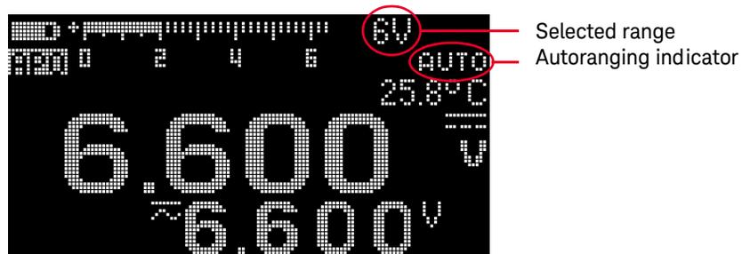
Pressing **Range** changes the tester range (and disables auto-ranging). Each additional presses of **Range** (in manual ranging) sets the tester to the next higher
