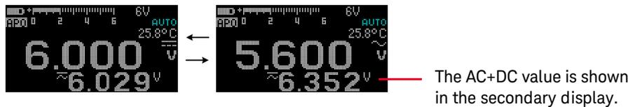
The **Auto** function identifies the signal component using the following rules:
