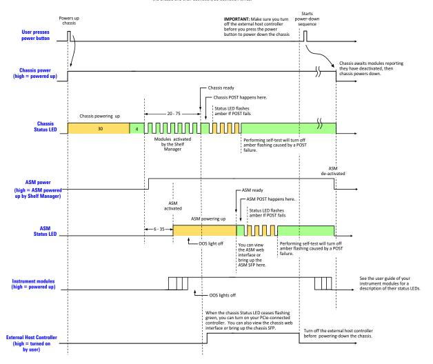
In brief, the host PC must be off whenever the chassis is powered up or down. Because modules are not hot-swappable, the chassis must be powered down before modules are added or removed.
