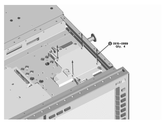
**NOTE:** It would be important to install the new Attenuator in to the bottom position (source 1) so the instrument could have Fast Tune capabilities.
