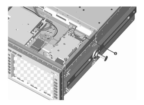
**STEP 13:** Re-install the shorting spring that you removed earlier. Tighten the 4 screws with a T-10 Torx driver to 9 in.lbs.
