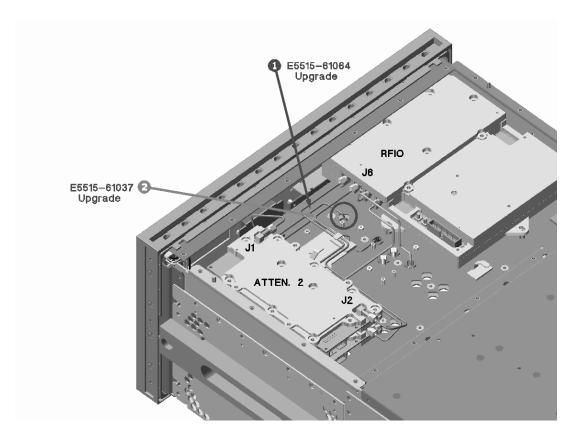
**STEP 10:** Attach the E5515-61064 cable to the input connector on the attenuator from the kit. Tighten the cable with a 5/16" wrench set too 9 in.lbs.
