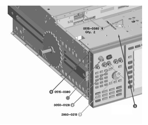
**STEP 1:** Remove the RF Interface module.
