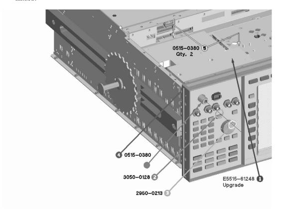
**STEP 15:** Attach all the cables to the RF Interface. Tighten the 4 semi-rigid cables with a 5/16" wrench to 9 in.lbs.
