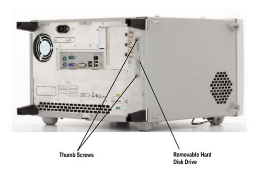
2 Pull the drive tray out to remove the disk drive.
