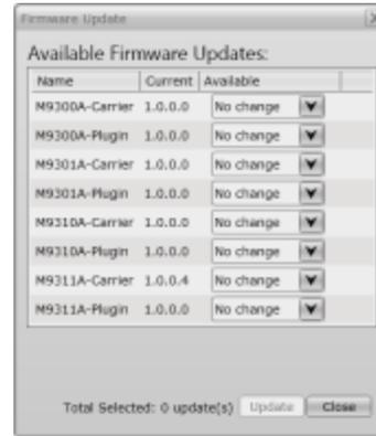
4. Close the **Firmware Update** dialog box if no firmware updates are necessary. If firmware updates are required, install the updates, shut down the computer, cycle power on the M9018A PXIe Chassis, and repeat this procedure to verify connection, perform self-test, and verify that no further firmware updates are necessary.
