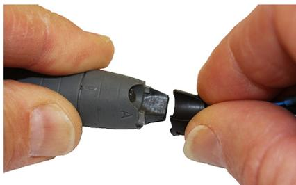
Figure 4 Aligning the Tip to the Probe
