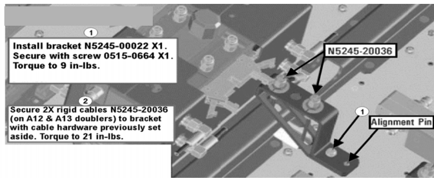
Figure 15 Cable Bracket Mount Installation (N5245-00022, 0515-0664, N5245-20036)
