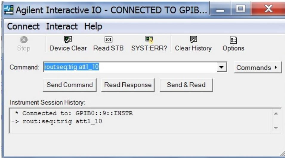
9. To confirm that the Connection Expert can control the Test Set, type the following command as shown in the Command field: **ROUT:SEQ:TRIG ATT1\_10** [Send Command]
