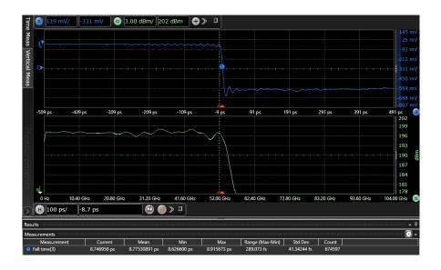
8.8ps edge is measured with InfiniiMax 4 probing solution with 52 GHz solder-in probe head
