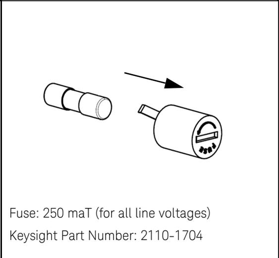
**3** Replace the fuse-holder assembly in the rear panel.
