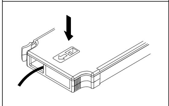
**5** Install the module into mainframe.
