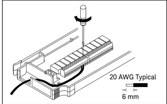
**3** Route wiring through strain relief.
