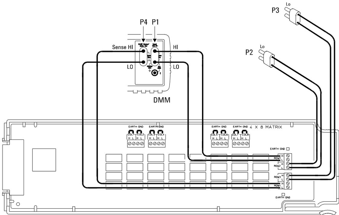
*Connections for 34904A Verification Tests*
