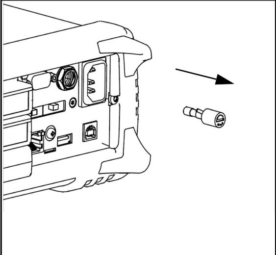
**2** Remove the fuse from the assembly.
