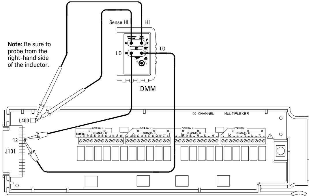
*Connections for 34908A Verification Test 1*
