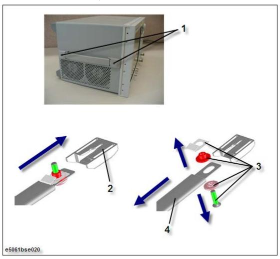
Replacement Procedure Handle Assembly Replacement Keysight E5061B Network Analyzers
