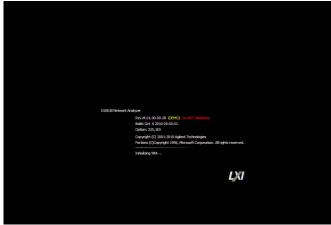
If the display whited out, entirely blued or appeared with a dialog box, a mass storage problem is suspected. Try to perform the mass storage recovery procedure.
