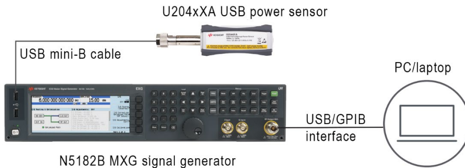
Figure 19. Connection diagram showing a USB power sensor connected to the N5182B MXG signal generator's USB port
