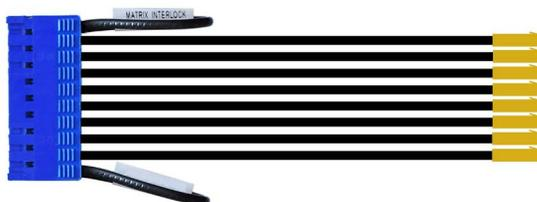
Four modules can be interconnected on each side of the mainframe in this manner, using three expansion cables. Should you need to make the last connection (between the two upper or lower modules) for an eight-module expanded matrix, you would have to fabricate the interconnection using eight 22 to 28 AWG wires, fitted to “crimp-to-wire” contacts with latch tabs.
