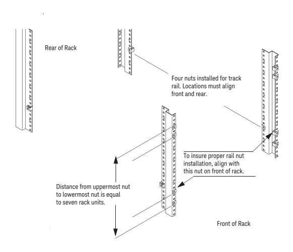
**6** Attach the track rails to the rack using the four 10–32 flat head screws and #2 Phillips screwdriver provided.
