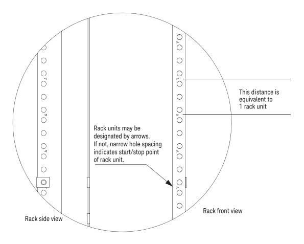
The following figure indicates proper locations for sheet metal nut locations. To ensure a level installation, the same seven rack unit locations are used on each vertical rack piece.
