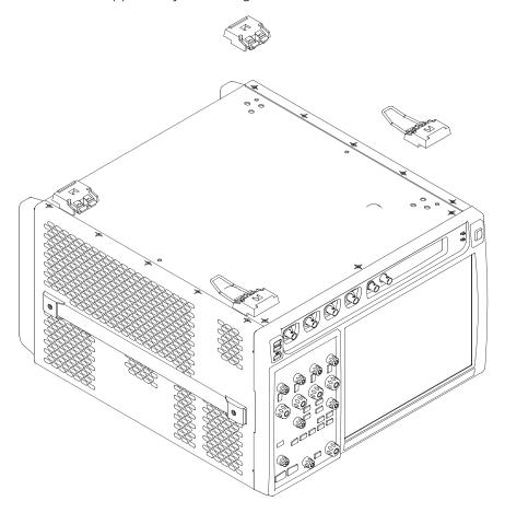
2 Grasp the feet firmly and squeeze the tab in the directions shown (1), slide (2), and lift off (3).
