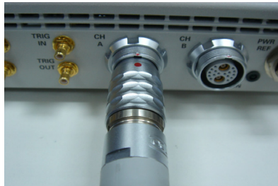
Figure 1-10 Connecting the P-Series power sensor
