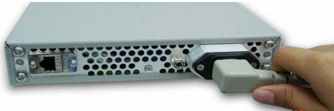
Figure 1-6 Connecting the power cord
