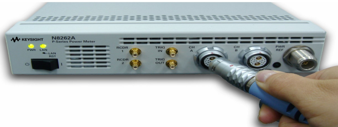
Figure 1-14 Connecting power sensor to CH A input connector
