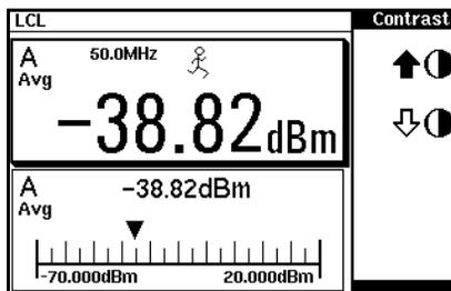
Figure shows display with an E-Series E9320 power sensor connected.
