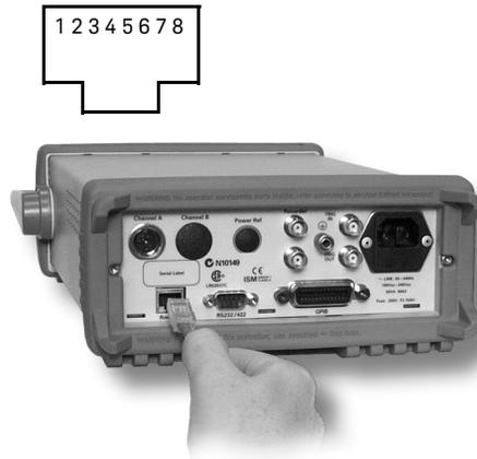
**4** Recorder output (two outputs are fitted to dual channel meters) and Trigger Input and Output connections are made via BNC connectors.
