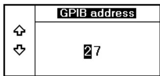
To ensure the GPIB interface is selected press **System**, **Remote Interface**, **Select Interface**, **GPIB**.
