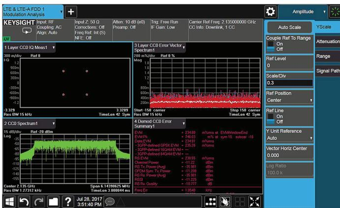
Figure 7b. 5 MHz E-TM 1.1 signal without baseband filter and symbol rolloff length = 20 Ts (best EVM).
