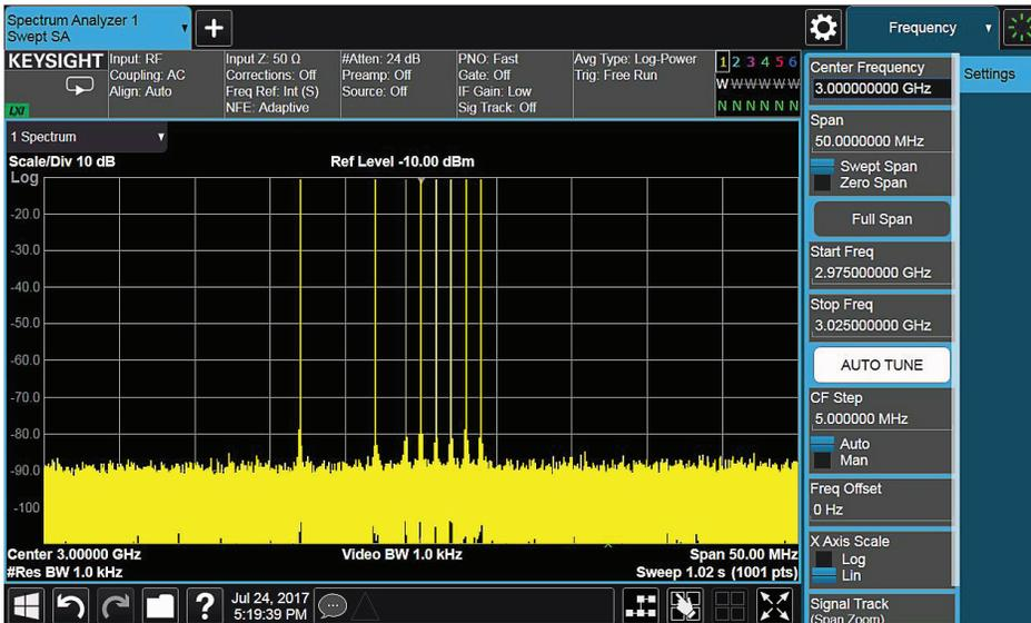
Figure 5d. Unequally spaced tones corrected with predistortion techniques.
