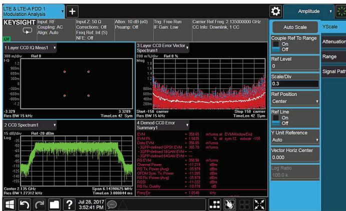
Figure 7c. 5 MHz E-TM 1.1 signal with baseband filter and symbol rolloff length = 20 Ts.
