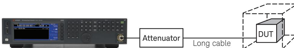
Figure 6b. When decreasing amplitude range, place your DUT in a shielded environment.
