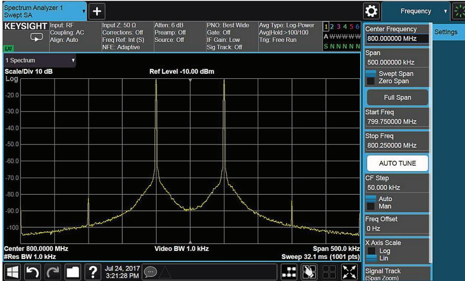
Figure 5c. Two tone signal created on a vector signal generator showing over 70 dBc from the two tones to the third-order products.
