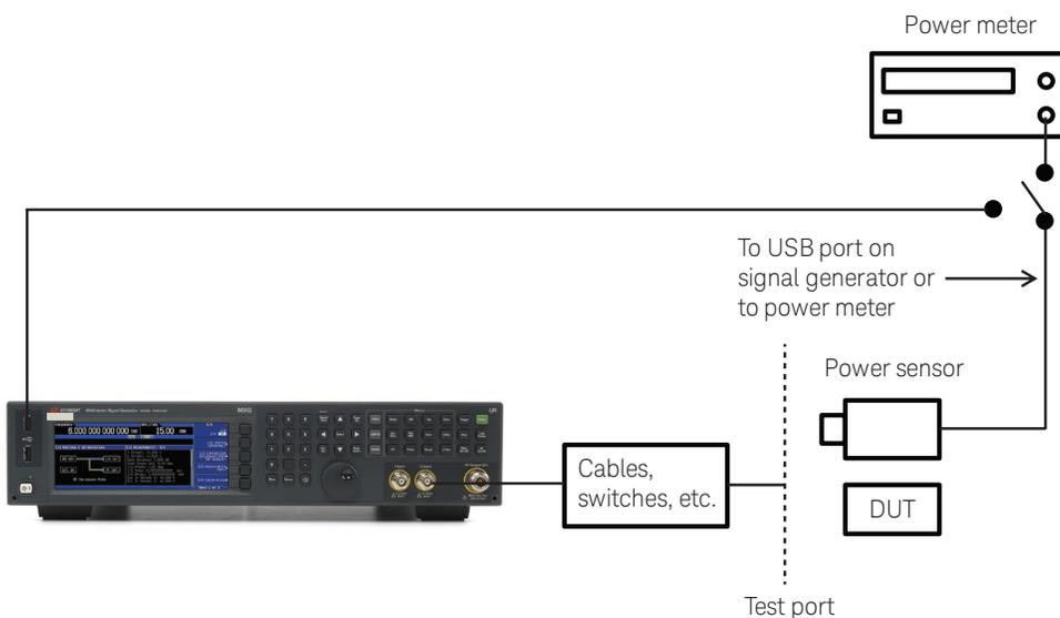
Figure 2. Setup for improving level accuracy of the signal.
