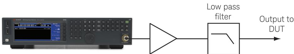
Figure 6a. When increasing amplitude range, use a low pass filter to reduce added harmonic distortion.
