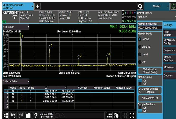
Figure 1a. Harmonic distortion measurement using a signal analyzer.
