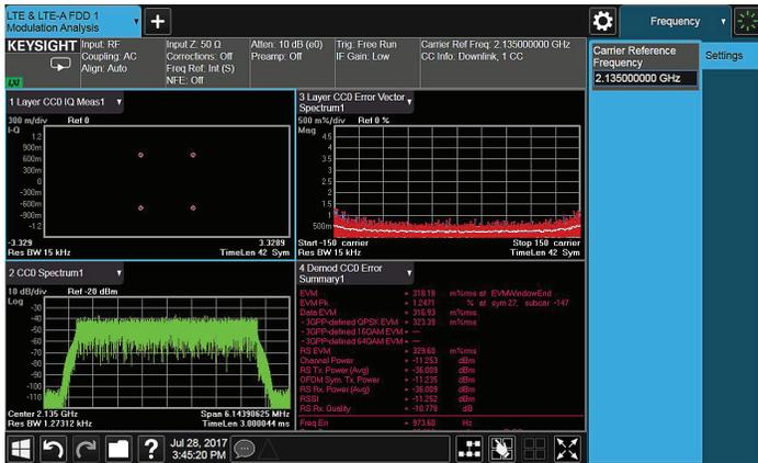
Figure 7a. 5 MHz E-TM 1.1 signal with default baseband filter (best ACLR).
