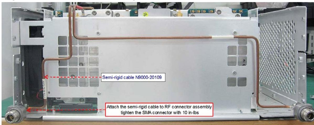
3. Refer to **Figure 10**, connect the other end of the cable (1) to tracking generator assembly. Tighten the SMA connector with 10 in-lbs.
