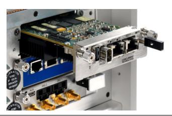
**5.** Attach retainer bracket in order to secure module in place.
