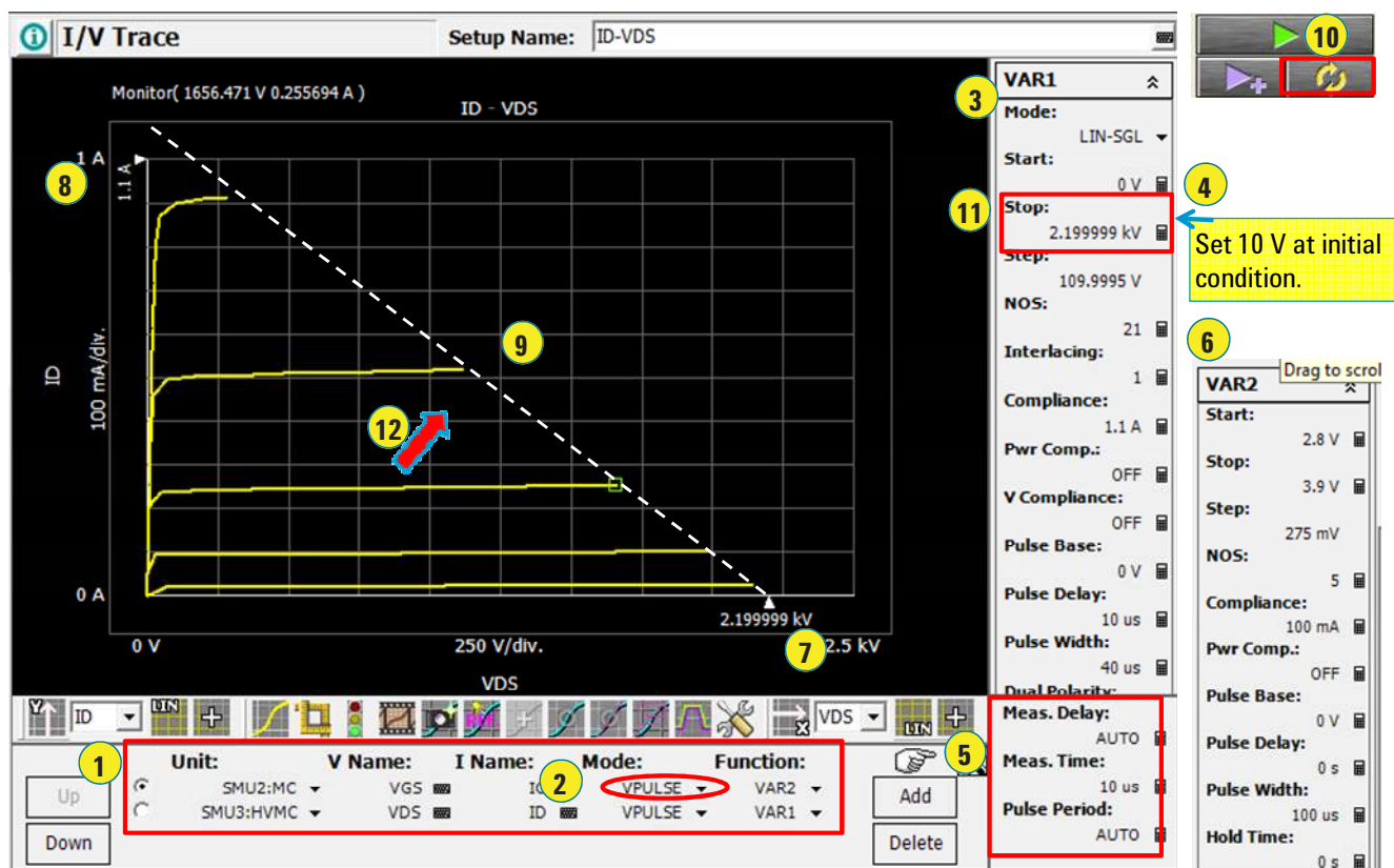
Figure 6-13. To setup 2.2 kV Tracer Test using HVMCU.
