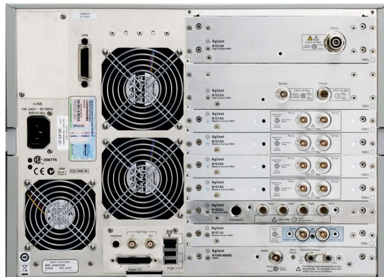
B1505A std. Demo configuration (back)
