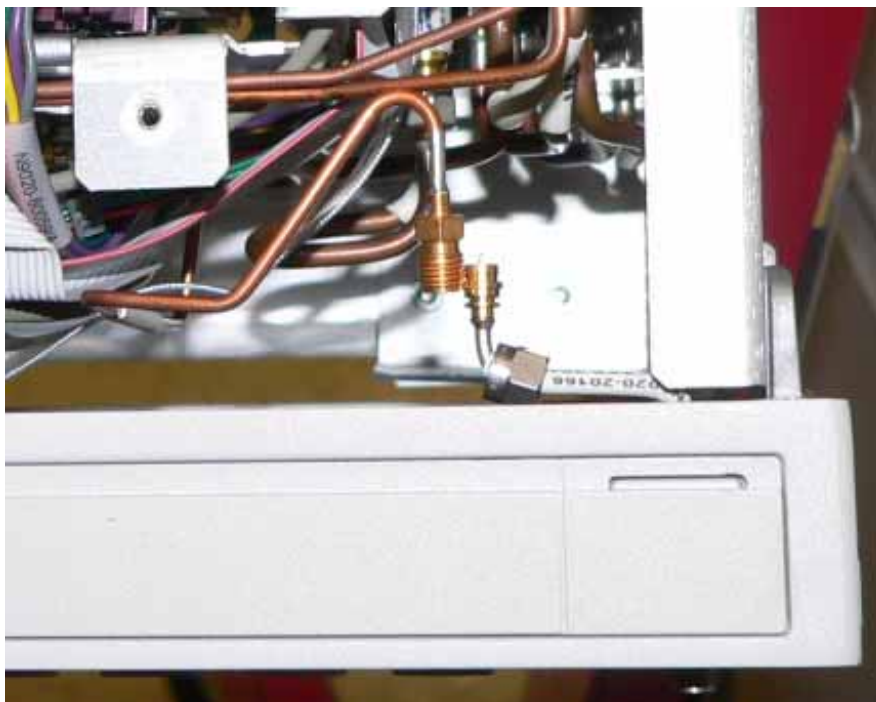
Figure 14 W17 and W29 Properly Aligned
