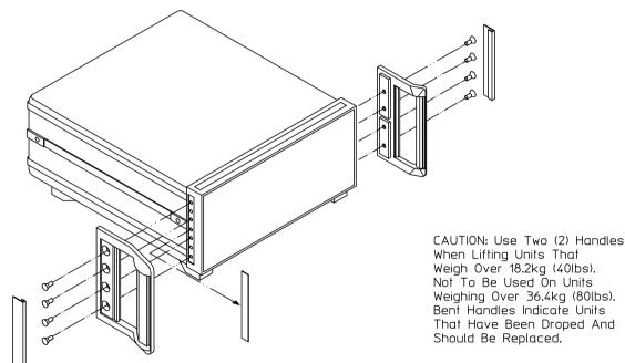
CAUTION: THIS KIT CONTAINS ONLY METRIC HARDWARE. IF INCH HARDWARE IS NEEDED ORDER INCH HARDWARE KIT #5062-4078. INSTRUMENTS WITH METRIC CABINETS HAVE THE WORD "METRIC" CAST ON TOP OF THE FRONT FRAME (UNDER THE TRIM).
