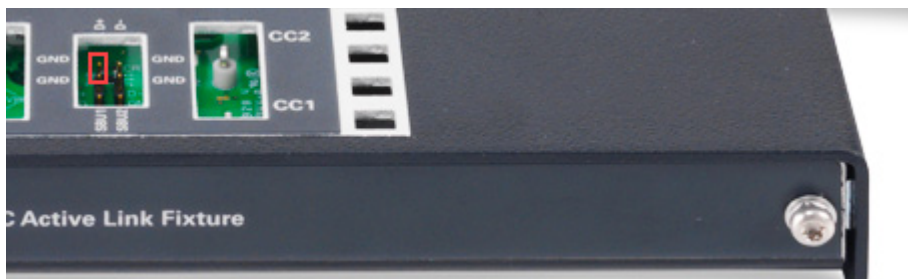
Figure 9 Top view of the N7019A highlighting the probe pins for probing D+ signal single-ended
