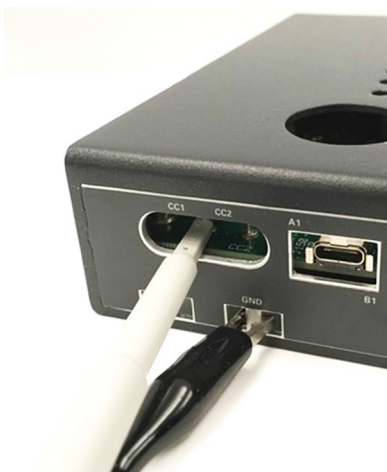
Figure 1 Probing the CC2 signal at the N7018A with the probe ground connected to the GND connection point
