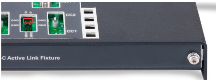
Figure 10 Top view of the N7019A highlighting the probe pins for probing D+ and D- signals differentially
