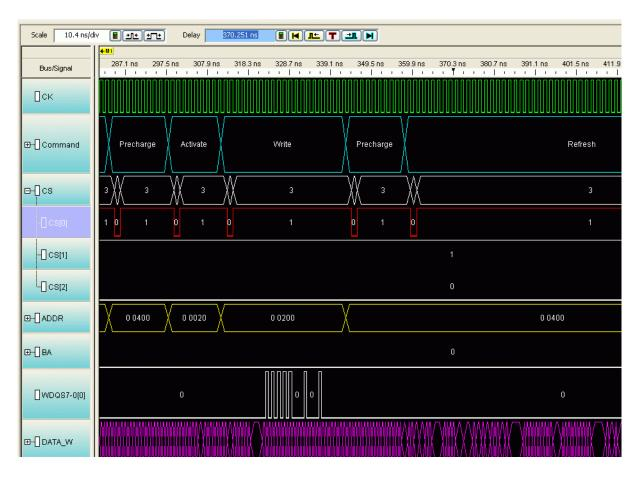
To check that all of the Write Data bits are aligned, configure the target to generate write-only traffic with an alternating 0/1 bit pattern. If necessary, select a different eye opening so that each DQ signal is sampled at the same time. In the following example, the first data bit needs to be adjusted:
