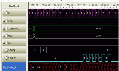
Once the read data sample positions are selected, find the correct sample for the DQS\_R signal. Utilize the waveform view of the state acquisition.
