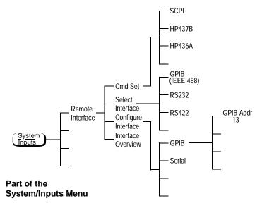
Check and, if required, change the address by pressing System Inputs,
