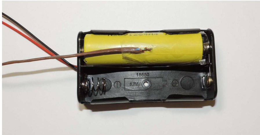
Figure 6 Attaching the thermocouple to the Cell-Under-Test
