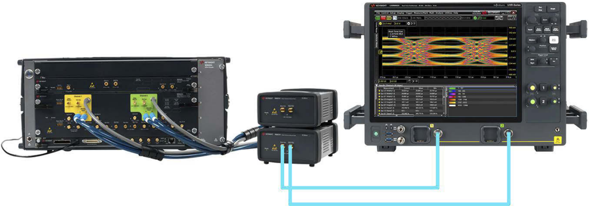
Figure 88 Amplitude Calibration connections for C2C and KR using UXR oscilloscope (2 channels)
