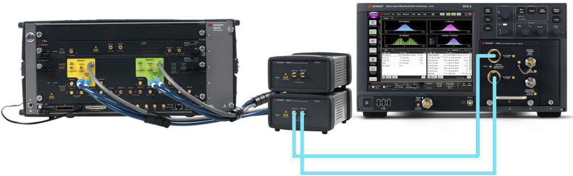
Figure 42 Amplitude Calibration connections for C2M Host and C2M Module using DCA-X oscilloscope and M8040A
