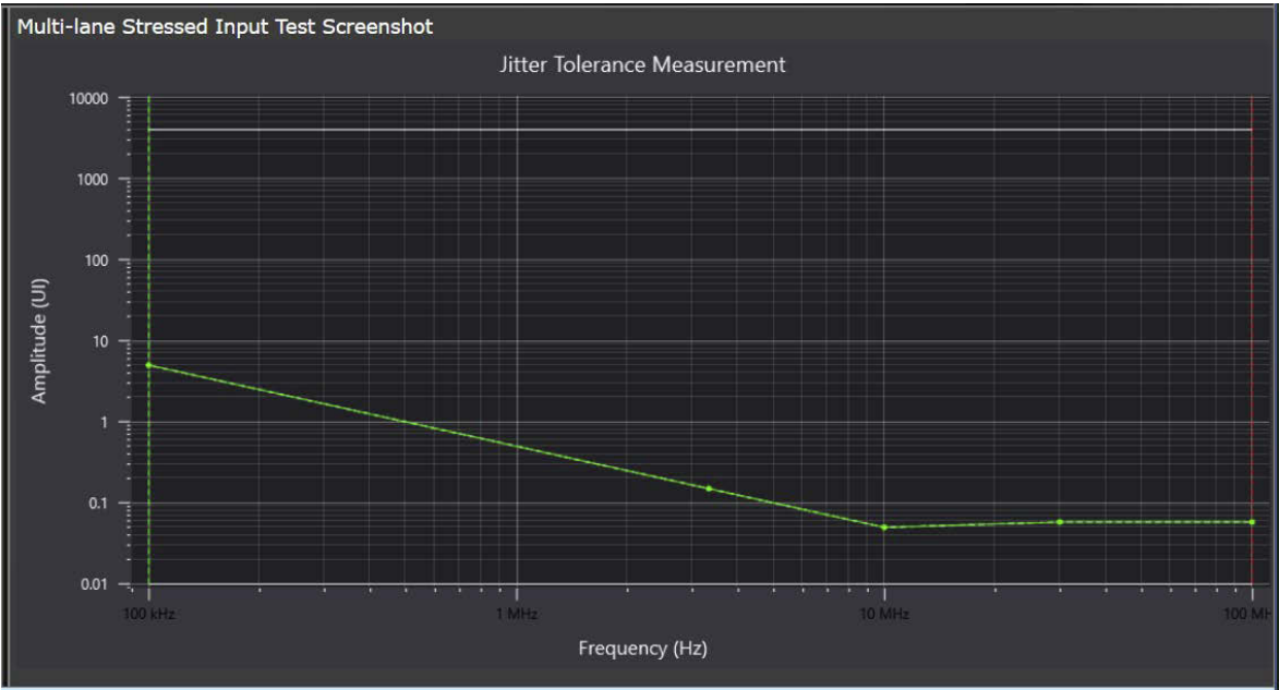
Figure 78 C2M Host Multi-lane Stressed Input Test Result (graphical)
