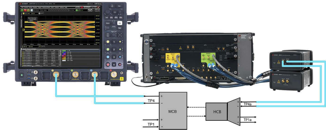
Figure 39 Crosstalk Calibration connections for C2M Module using UXR oscilloscope (4 channels) and M8040A
