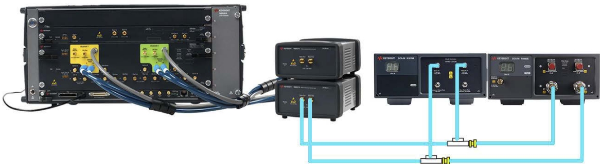
Figure 87 Amplitude Calibration connections for C2C and KR using DCA-M oscilloscope and M8040A
