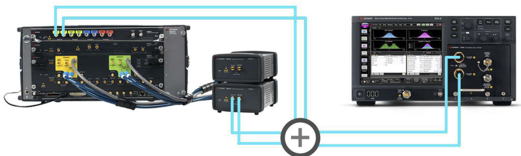
Figure 90 Amplitude Calibration connections for CR (M8040A)
