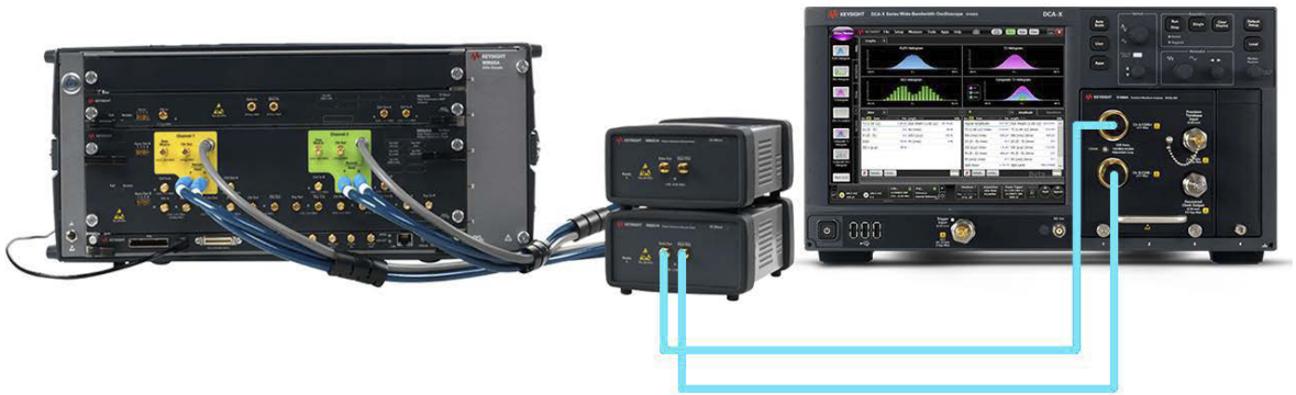
Figure 86 Amplitude Calibration connections for C2C and KR using DCA-X oscilloscope and M8040A
