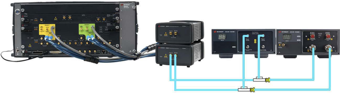
Figure 43 Amplitude Calibration connections for C2M Host and C2M Module using DCA-M oscilloscope and M8040A
