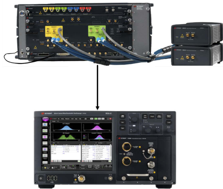
Figure 28 COM procedure: Schematic test setup for equipment calibration and Tx characterization
