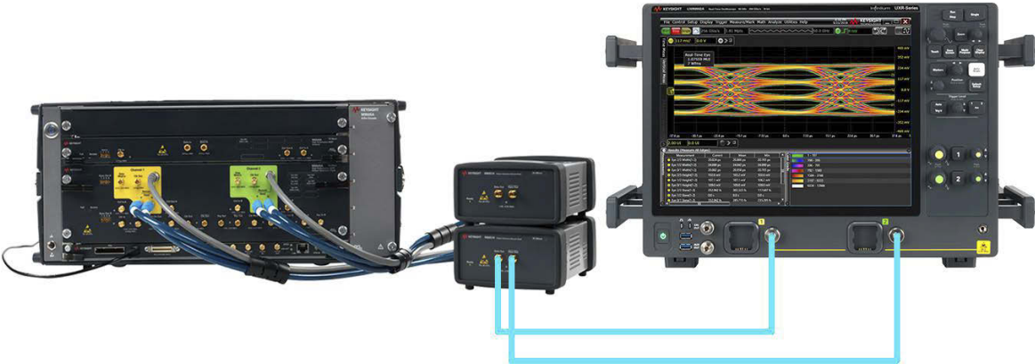
Figure 44 Amplitude Calibration connections for C2M Host and C2M Module using UXR oscilloscope (2 channels)
