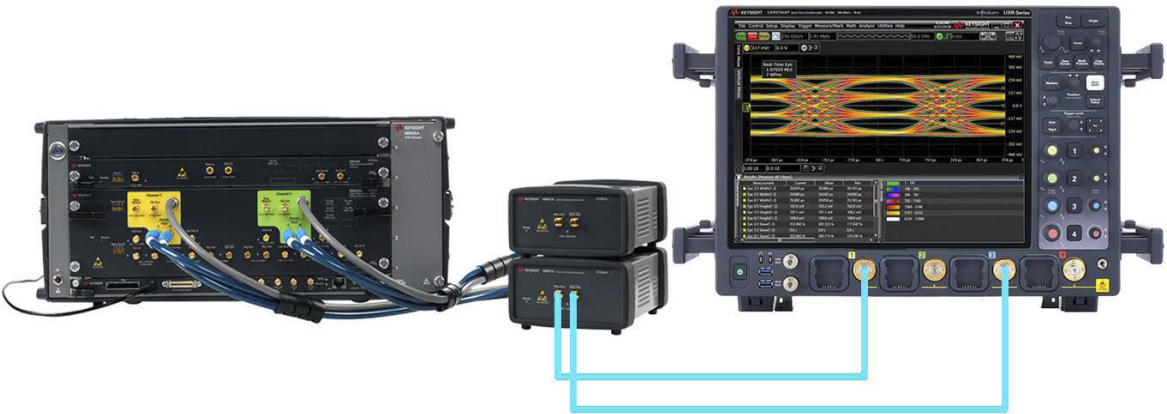
Figure 89 Amplitude Calibration connections for C2C using UXR oscilloscope (4 channels)
