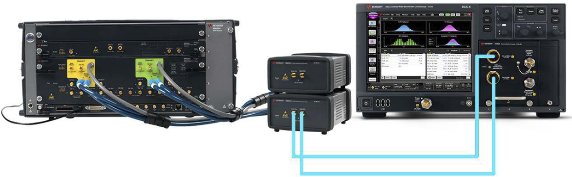
Figure 109 Connections for Peak to Peak Amplitude Calibration for ATol for CR (M8040A)
