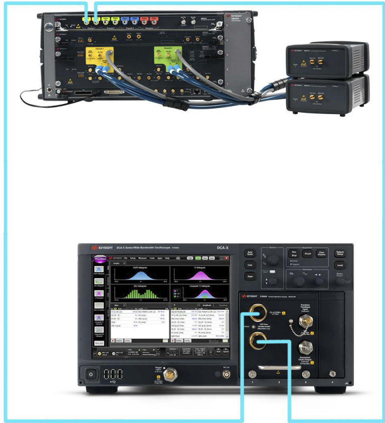
Figure 98 Broadband Noise Calibration connections for C2C and KR (M8040A)
