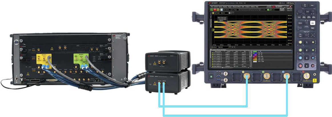
Figure 45 Amplitude Calibration connections for C2M Host and C2M Module using UXR oscilloscope (4 channels)
