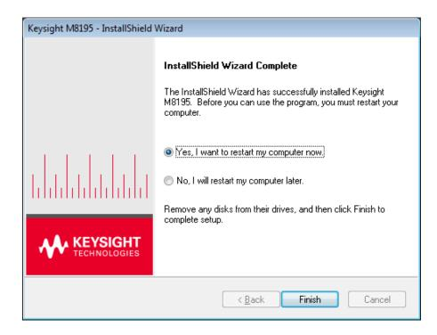
15. Click **Finish** to restart your system. Do not connect the AXIe chassis to your system using the PCIe or USB cable during this reboot.
