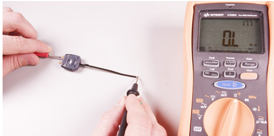
Figure 23 Resistance measurement for a damaged MX0100A probe head
