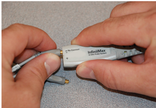
Figure 4 Properly Pulling the Probe Head Straight Out
