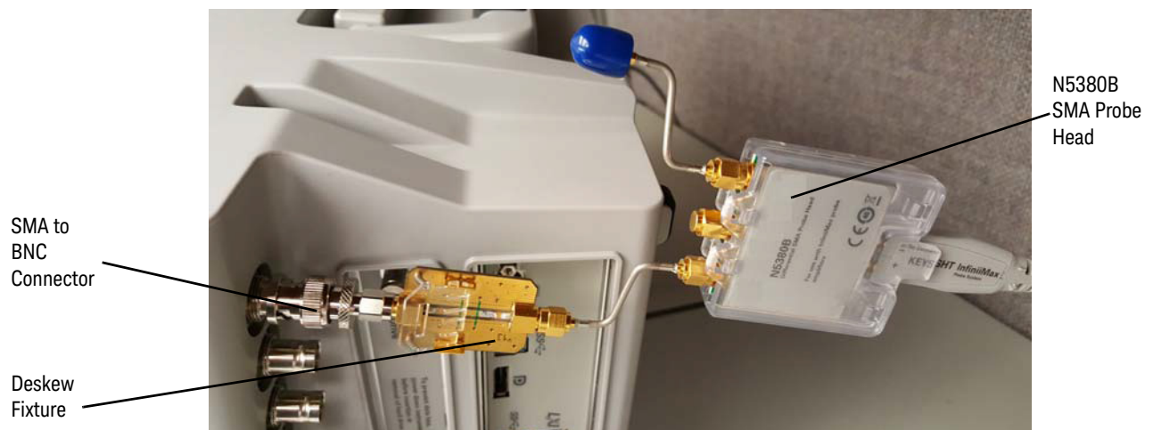
Figure 55 Connecting the SMA Probe Head and Deskew Fixture
