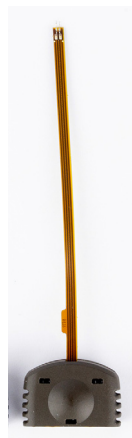
Discoloration after usage under high temperatures
