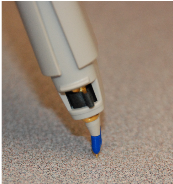
Figure 28 Proper Vertical Orientation of the Blue Tips
